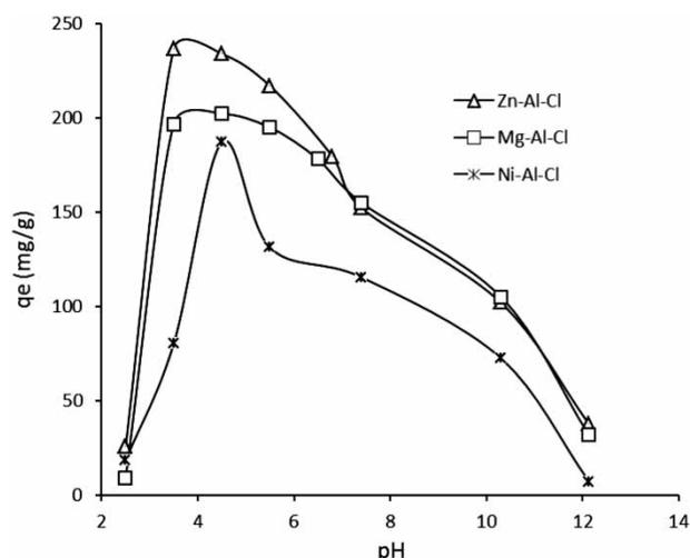
**Figure 5** | Effect of solution pH on MO removal (adsorbent dose: 80 mg/L, contact time: 8 h, initial MO concentration: 20 mg/L, temperature: 25 °C and agitation speed 500 rpm).
