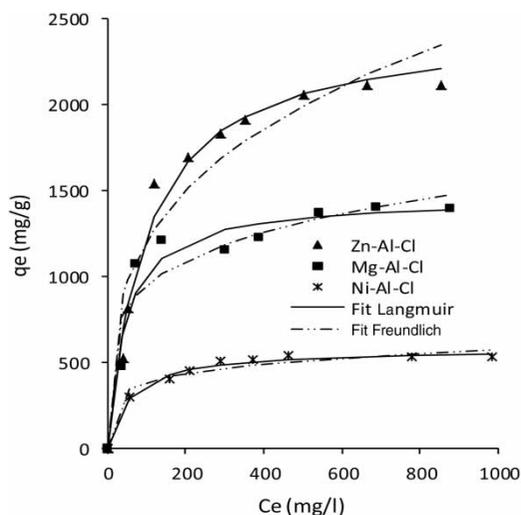
**Figure 7** | Adsorption isotherms of MO onto LDHs (adsorbent dose: 80 mg/L, pH: 8, contact time: 8 h, temperature: 25 °C and agitation speed: 500 rpm).
