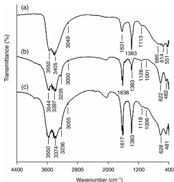
Figure 3 | FTIR spectra of (a) Zn-Al-Cl, (b) Mg-Al-Cl and (c) Ni-Al-Cl.
