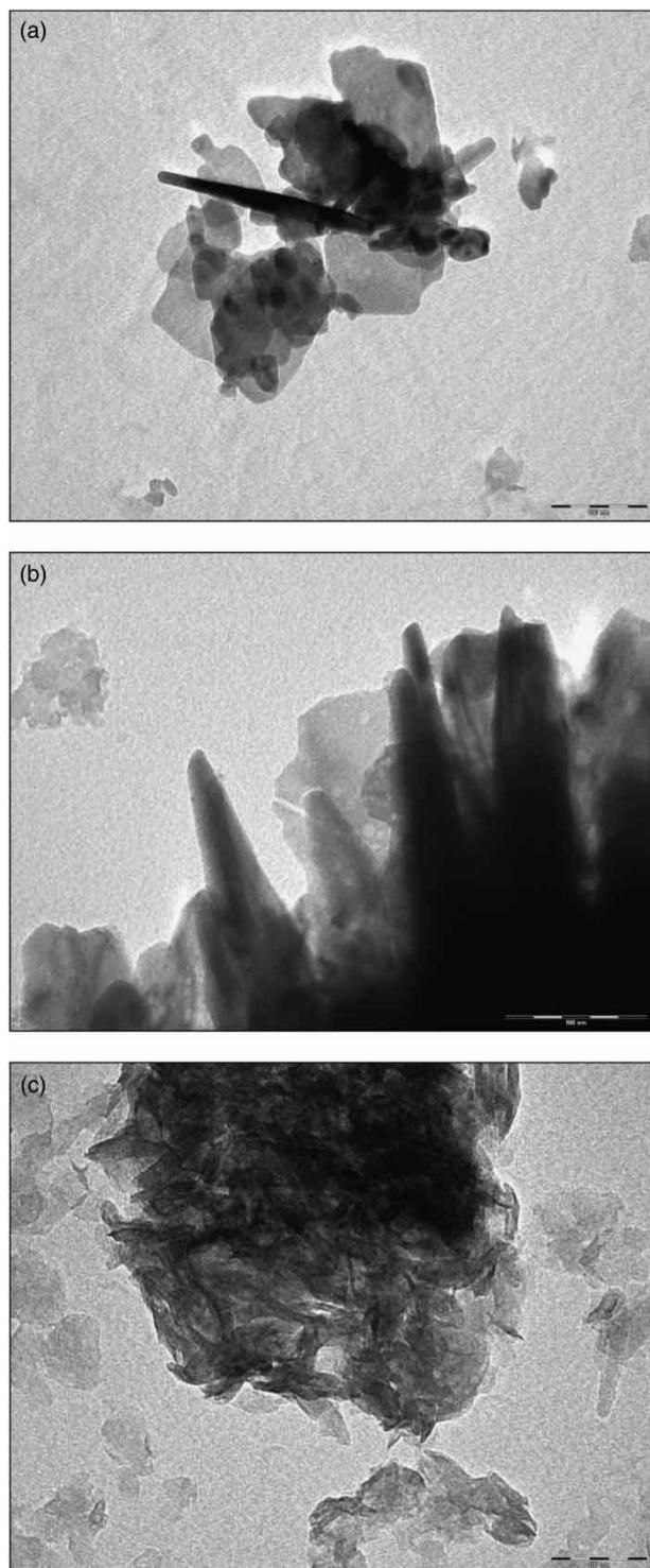
**Figure 4** | TEM micrographs of the LDH samples: (a) Zn-Al-Cl, (b) Mg-Al-Cl and (c) Ni-Al-Cl.
