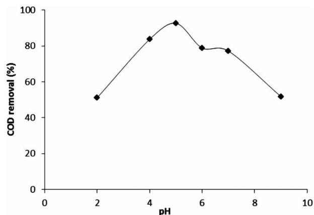
**Figure 8** | Effect of pH on COD removal by Zn-Al-Cl ( $V = 20$  mL, Agitation speed: 500 rpm, contact time: 8 h and adsorbent dose: 1 g/L).
