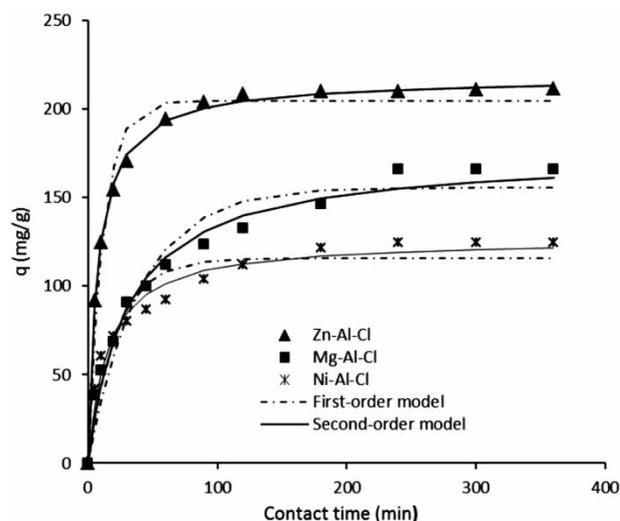
**Figure 6** | Effect of contact time and kinetic models of MO adsorption (adsorbent dose: 80 mg/L, initial MO concentration: 20 mg/L, temperature: 25 °C, agitation speed 500 rpm and solution pH: 8).
