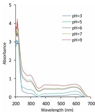
**Figure 9** | Variation in UV-Vis spectra of TWW treated by Zn-Al-Cl at different pH solution ( $V = 20$  mL, Agitation speed: 500 rpm, contact time: 8 h, adsorbent dose: 1 g/L).
