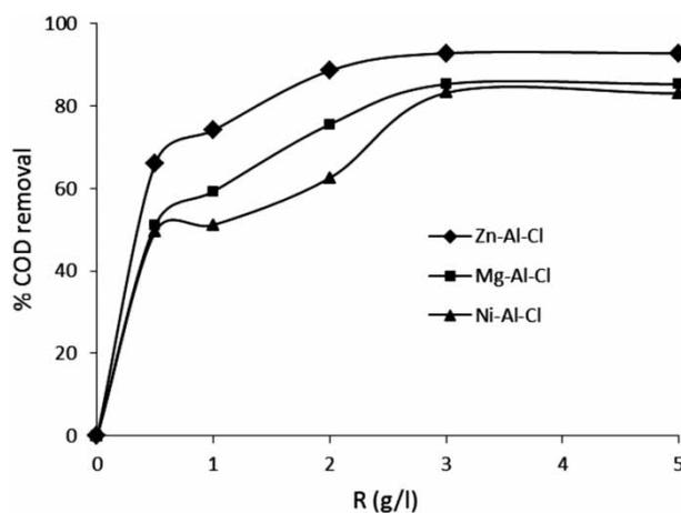
**Figure 11** | Effect of adsorbent dosage on COD removal by LDHs (pH 5, V = 20 mL and contact time: 8 h).
