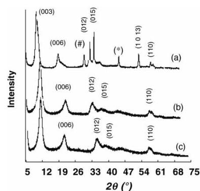
**Figure 1** | XRD patterns of (a) Zn-Al-Cl, (b) Mg-Al-Cl and (c) Ni-Al-Cl, (\*) Zn(OH)<sub>2</sub> and (#) Al(OH)<sub>3</sub>.
