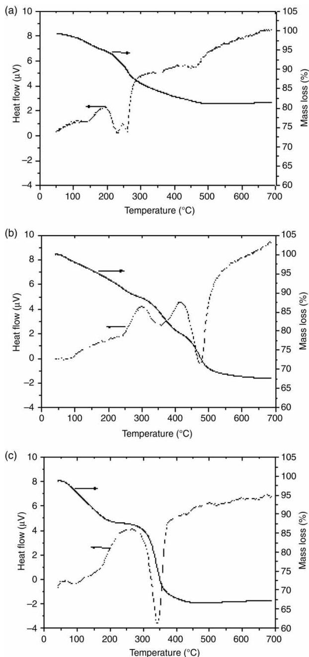
**Figure 2** | TGA-DTA curves of Zn-Al-Cl (a), Mg-Al-Cl (b) and Ni-Al-Cl (c).
