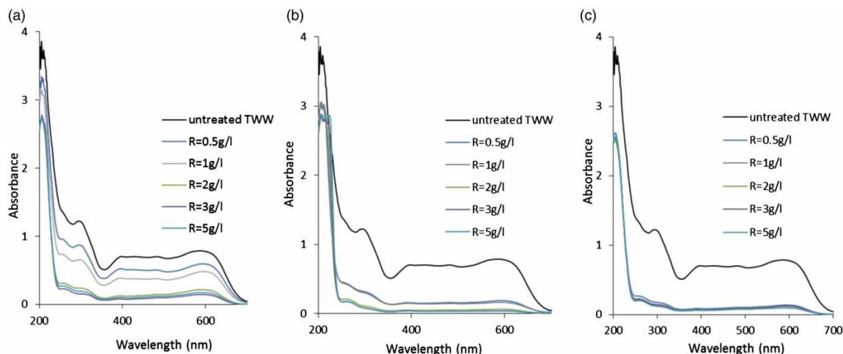
**Figure 10** | Variation in UV-Visible spectra of TWW at different LDH dosages: (a) Zn-Al-Cl, (b) Mg-Al-Cl and (c) Ni-Al-Cl (pH = 5, V = 20 mL and contact time: 8 h).
