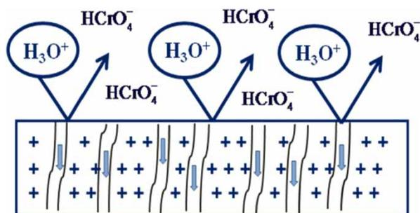
Figure 9 | Schematic representation of chromium ion repulsion.
