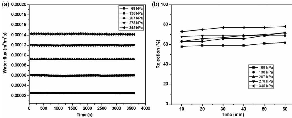
**Figure 7** | Effect of applied pressure on (a) permeate flux and (b) removal (%) for the MFI membrane (applied pressure: 69–345 kPa; cross flow rate:  $1.11 \times 10^{-6} \text{ m}^3/\text{s}$ ; feed concentration: 1,000 ppm).
