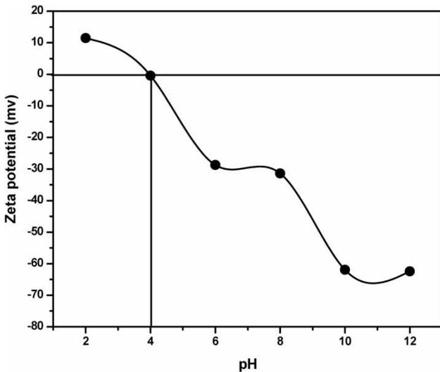
**Figure 8** | Zeta potential measurement of MFI zeolites at various pH.
