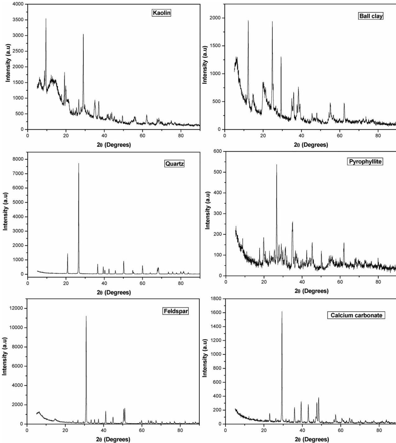
Figure 3 | XRD patterns of the raw materials used for the preparation of the substrate.
