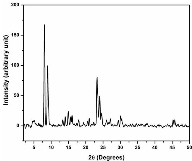
**Figure 4** | XRD analysis of MFI zeolite.
