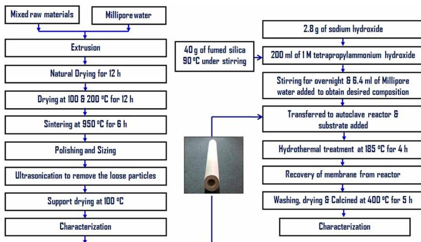
Figure 1 | Preparation of MFI zeolite membrane.
