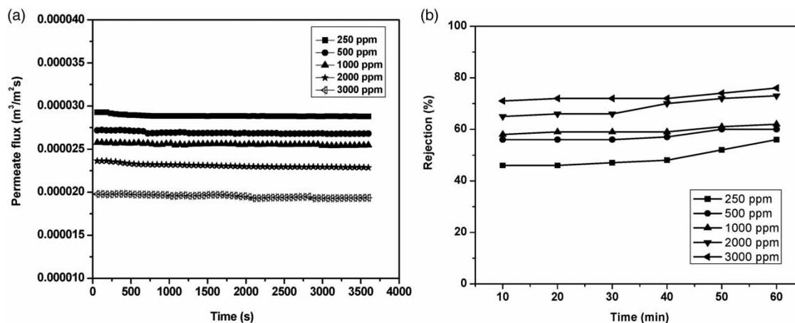
Figure 10 | Effect of initial feed concentration on (a) permeate flux and (b) removal (%) for the MFI membrane (feed concentration: 250–3,000 ppm; applied pressure: 69 kPa; cross flow rate:  $1.11 \times 10^{-6} \text{ m}^3/\text{s}$ ).
