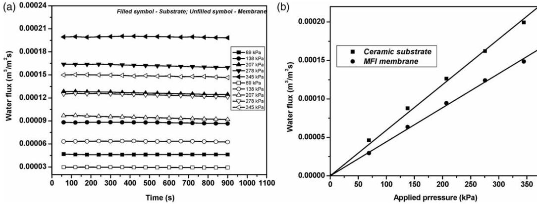
**Figure 6** | (a) Water flux as a function of time for pressures and (b) water flux as a function of applied pressure for the ceramic substrate and zeolite membrane.
