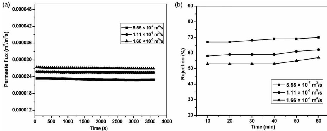
**Figure 11** | Effect of cross flow rate on (a) permeate flux and (b) removal (%) for MFI membrane (cross flow rate:  $5.55 \times 10^{-7}$ – $1.66 \times 10^{-6}$  m<sup>3</sup>/s; applied pressure: 69 kPa; feed concentration: 1,000 ppm).
