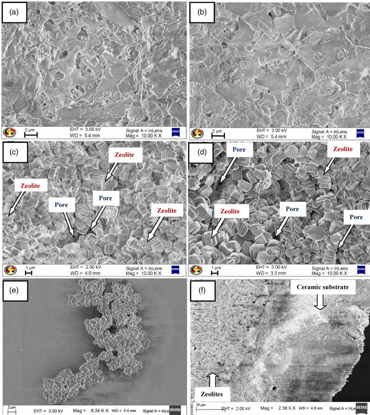
**Figure 5** | (a) and (b) FESEM images of the inner and outer surfaces of the substrate; (c) and (d) inner and outer surfaces of the MFI zeolite membrane; (e) MFI zeolite particles; and (f) cross-sectional view of the MFI zeolite membrane.
