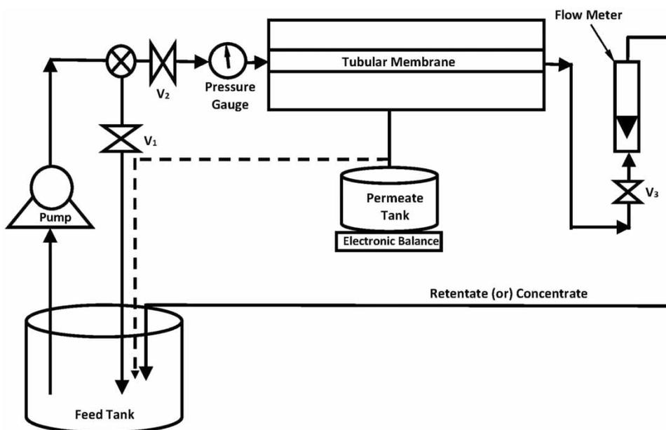
Figure 2 | Schematic of experimental setup ( $V_1$ -by-pass valve,  $V_2$ -inlet valve,  $V_3$ -retentate valve).
