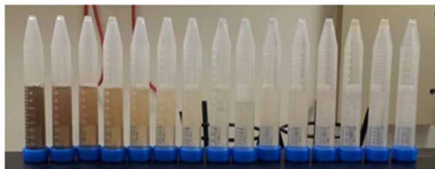
Figure 3 | Discoloration of sample A during electrolysis with BDD anode.
