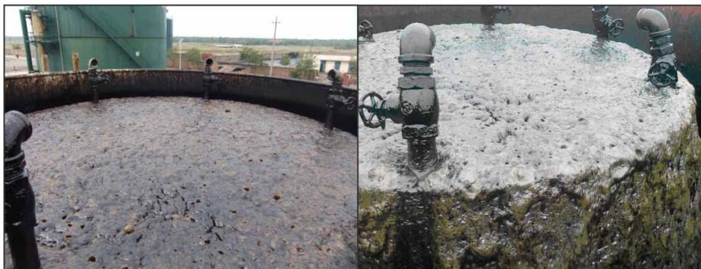
Figure 13 | Oil-bubble complexes of column 1 and oil-coal-bubble complexes of column 2.
