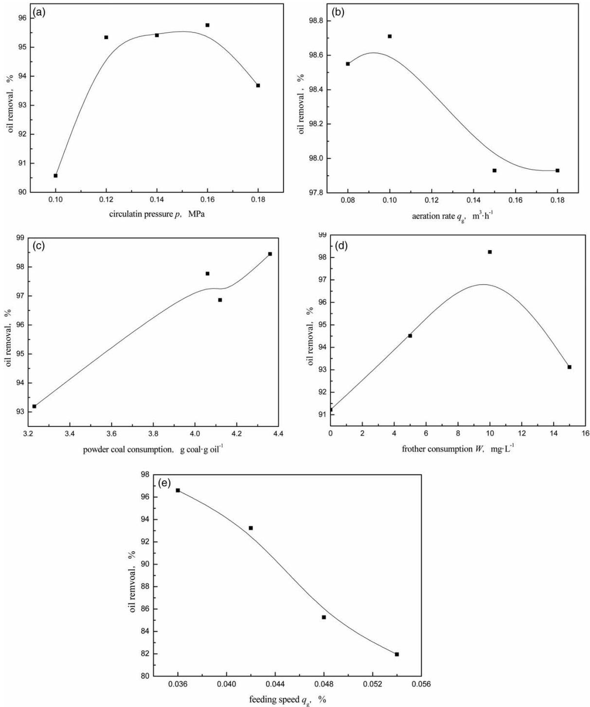
**Figure 8** | The operational parameters impact on the oil/water separation efficiency.
