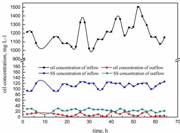
Figure 10 | The results of the  $30 \text{ m}^3 \text{ d}^{-1}$  oil-water separation experiment.
