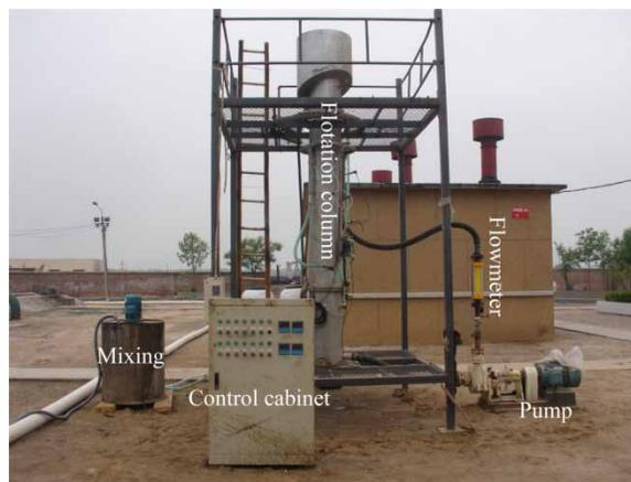
Figure 4 | 30 m<sup>3</sup> d<sup>-1</sup> Oil-water separation experimental system.
