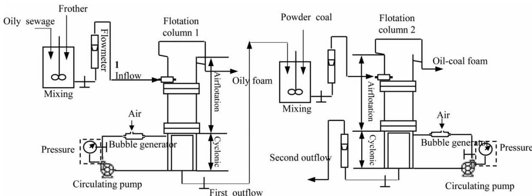
**Figure 6** | The combined process of coalescence-airflotation-carrier preferential adsorption.
