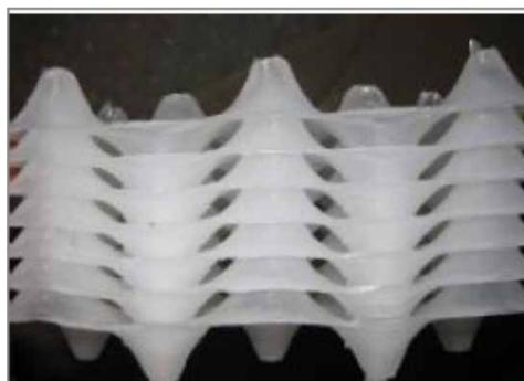
Figure 5 | Coalescent pack of flotation column.
