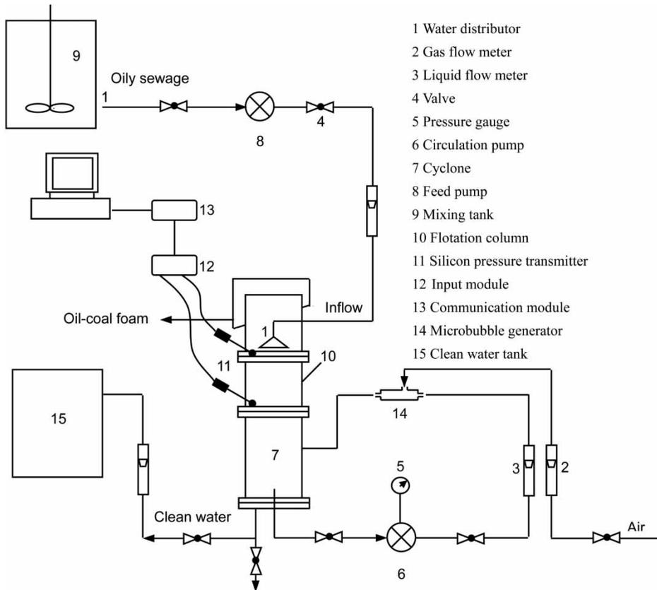
**Figure 2** | The diagram of experimental equipment connections.
