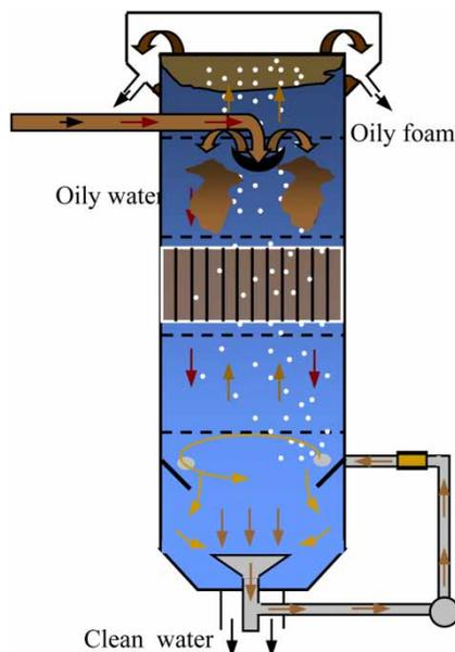
**Figure 1** | Cyclone-static microbubble flotation column (ZL 201020164545.3). Please refer to the online version of this paper to see this figure in color: <http://dx.doi.org/10.2166/wrd.2017.090>.
