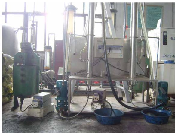
Figure 3 | 1 m<sup>3</sup> d<sup>-1</sup> Oil-water separation experimental system.
