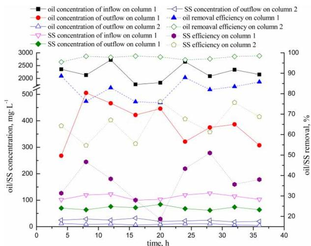
Figure 12 | Results of coalescence-airflotation-carrier preferential adsorption process experiment.
