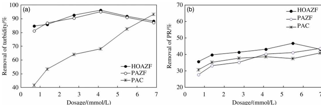
**Figure 5** | Impact of dosage on removal of phosphorus and turbidity with HOAZF and PAZF in treating a simulated pesticide wastewater. TP = 664.8–676.3 mg/L.
