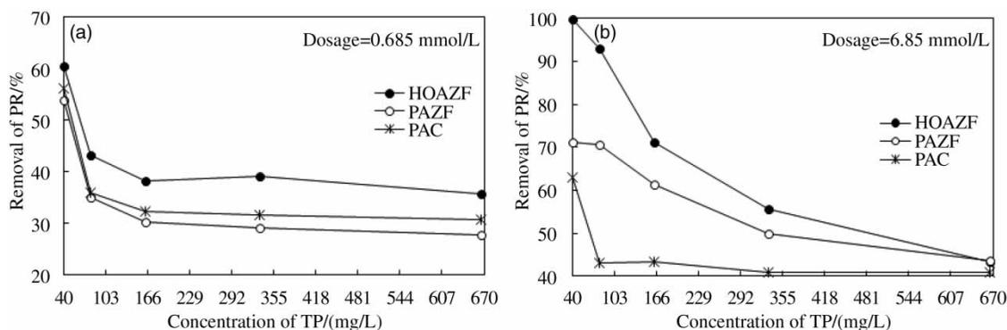
**Figure 7** | Impact of phosphorus level on removal of phosphorus and turbidity with HOAZF and PAZF in treating a simulated pesticide.
