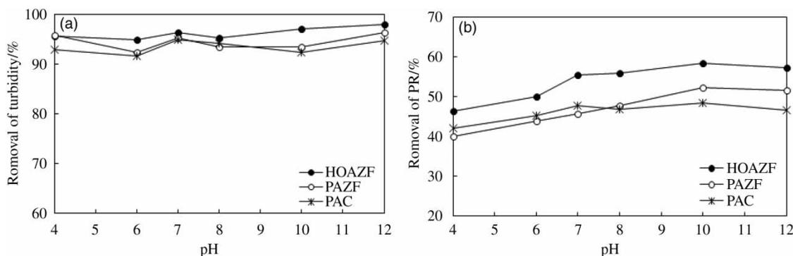
Figure 6 | Impact of coagulation pH on removal of phosphorus and turbidity by HOAZF and PAZF in treating a simulated pesticide wastewater. Dosage = 4.11 mmol/L.
