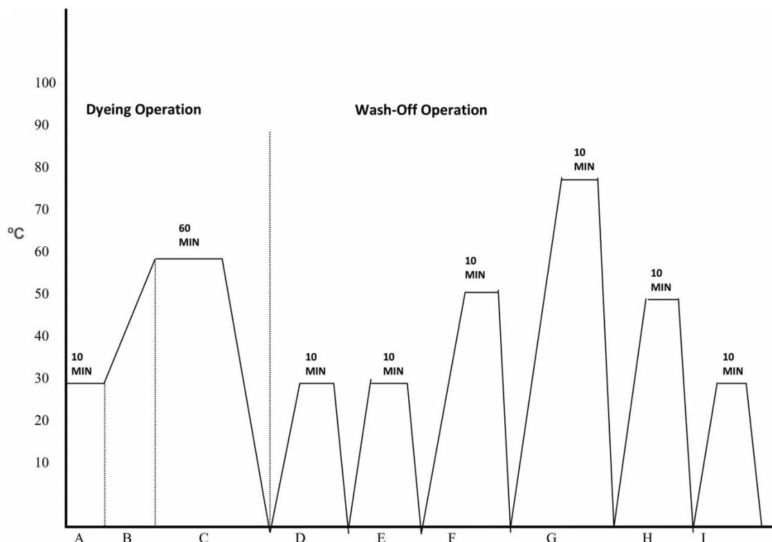
**Figure 1** | Isothermal dyeing process. A: Cold dyeing; B: Salt addition; C: Sodium carbonate addition and stirring for 45 minutes; D: Wash-off – Cold rinse; E: Neutralization wash with acetic acid; F: Warm wash; G: Soaping; H: Hot rinse; I: Cold rinse.
