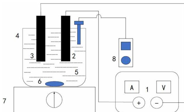
**Figure 1** | Electrocoagulation equipment (1. Power source; 2. parallel anode; 3. parallel cathode; 4. electrocoagulation cell; 5. electrolysis solution; 6. magnetic bar stirrer; 7. magnetic stirrer; 8. pH meter).
