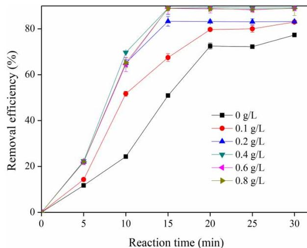
**Figure 3** | Effect of RSAC dosage on sulphate removal efficiency (conditions: reaction time 30 min; current density 70 mA/cm<sup>2</sup>; initial pH 6.5).
