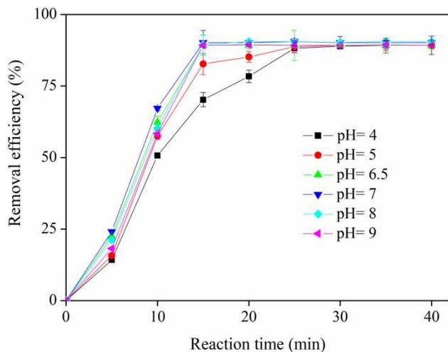
**Figure 4** | Effect of initial pH on the sulphate removal efficiency (conditions: current density 70 mA/cm<sup>2</sup>; RSAC dosage 0.4 g/L; reaction time 40 min).
