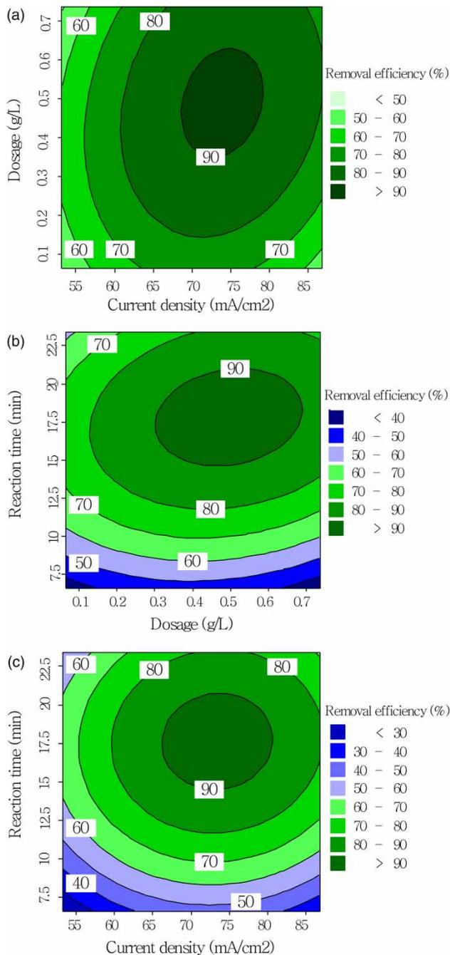
**Figure 5** | Response surface plots for interactive effect among factors ((a)–(c): current density and RSAC dosage; reaction time and RSAC dosage; current density and reaction time) on sulphate removal efficiency.
