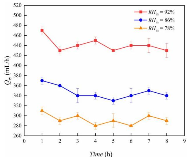
**Figure 6** | Water production rate of 8-hour continuous tests.
