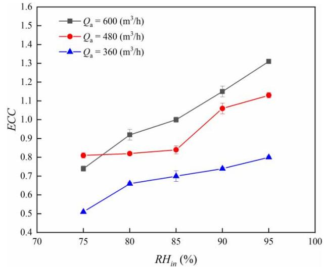
**Figure 13** | Variation of the energy conversion coefficient  $ECC$  with the air flow rate  $Q_a$ .
