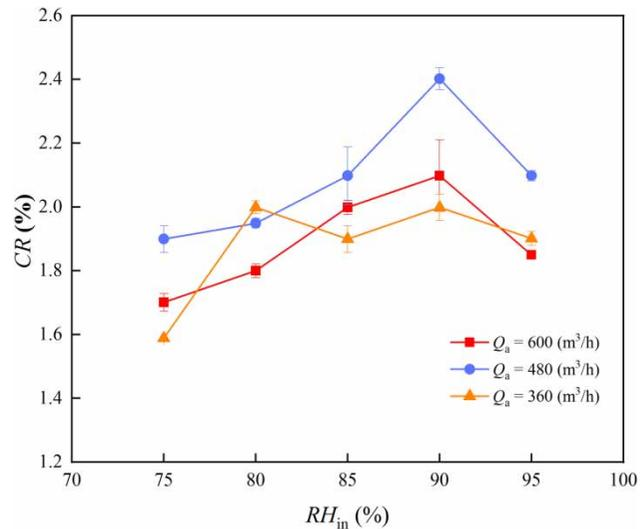
**Figure 14** | Variation of the condensing ratio  $CR$  with the air flow rate  $Q_a$ .
