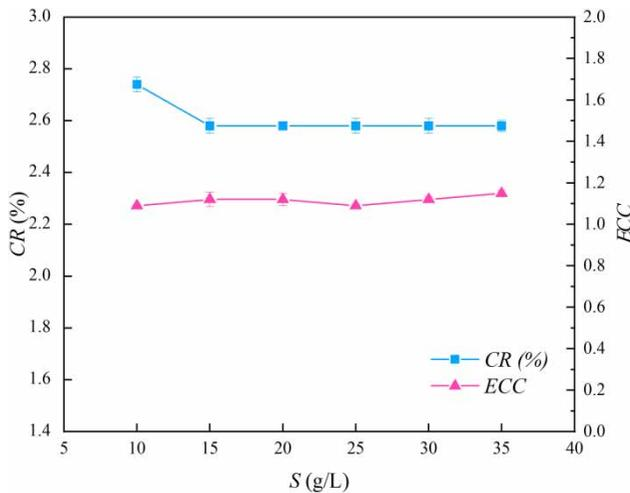
**Figure 16** | Influence of salinity of feed water  $S$  on the energy conversion coefficient  $ECC$  and the condensing ratio  $CR$ .
