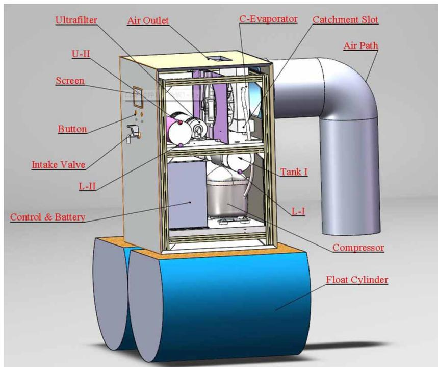
Figure 3 | 3-D model of the prototype.
