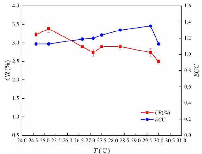
Figure 10 | Variation of the energy conversion coefficient  $ECC$  and the condensing ratio  $CR$  with the temperature of air flow at inlet  $T_{in}$ .
