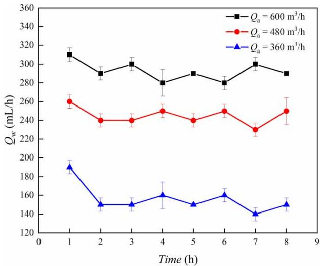
**Figure 12** | Variation of the water production rate  $Q_w$  with the air flow rate  $Q_a$ .
