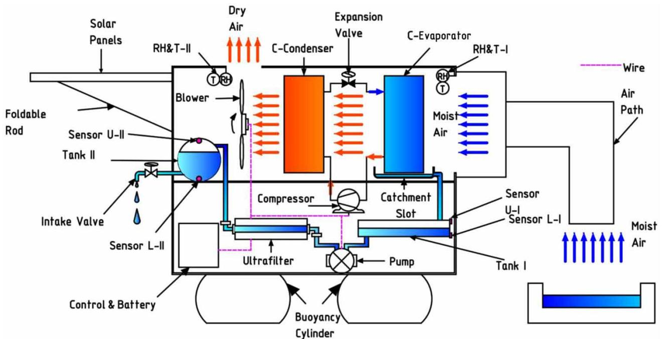
Figure 2 | Schematic diagram of the proposed AWG device.
