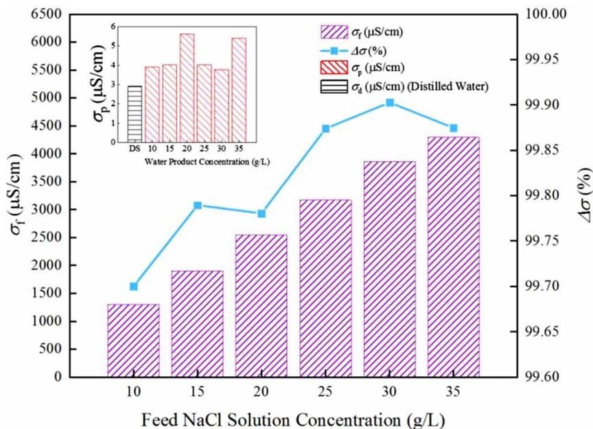
**Figure 8** | Electrical conductivity of the feed NaCl solution and the water product.
