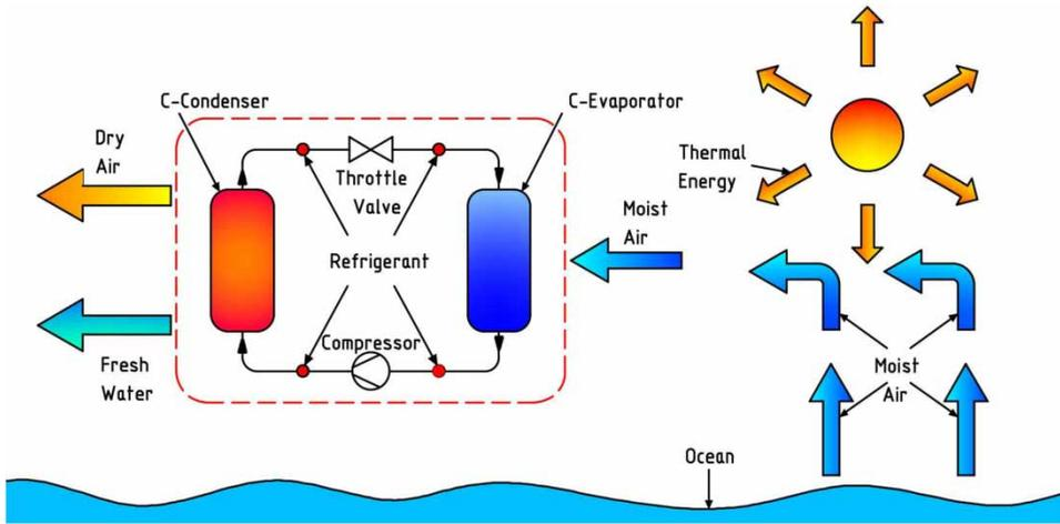
Figure 1 | Working principle of the AWG.
