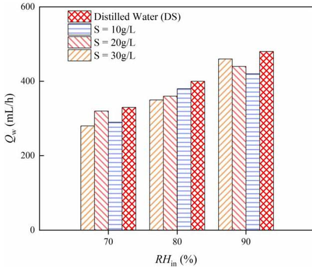
**Figure 15** | Influence of salinity of feed water  $S$  on the water production rate  $Q_w$ .
