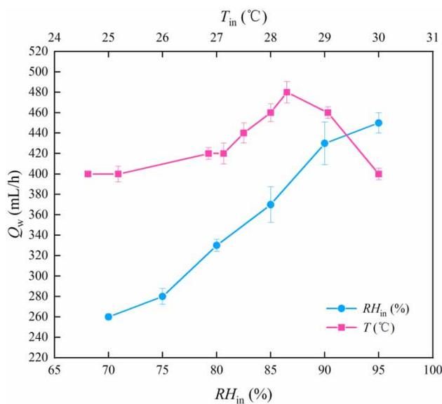
Figure 9 | Variation of water production rate  $Q_w$  with the temperature and relative humidity of air flow at inlet  $T_{in}$  and  $RH_{in}$ .
