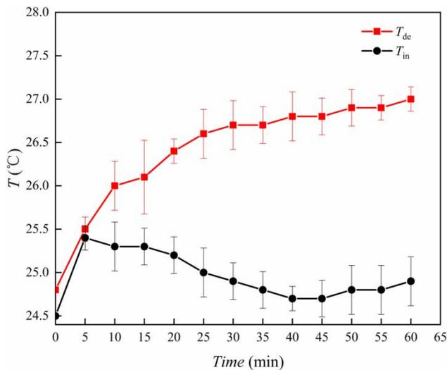
**Figure 7** | Variation of the temperature in the device  $T_{de}$  and the temperature of air flow at inlet  $T_{in}$  during the first hour.
