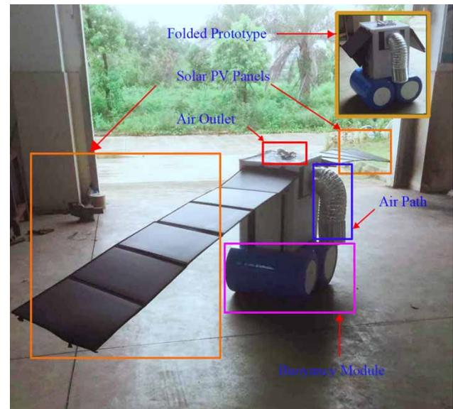
Figure 4 | Photographs of the prototype.
