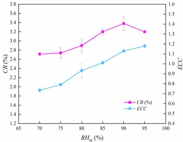
**Figure 11** | Variation of the energy conversion coefficient  $ECC$  and the condensing ratio  $CR$  with the relative humidity of air flow at inlet  $RH_{in}$ .
