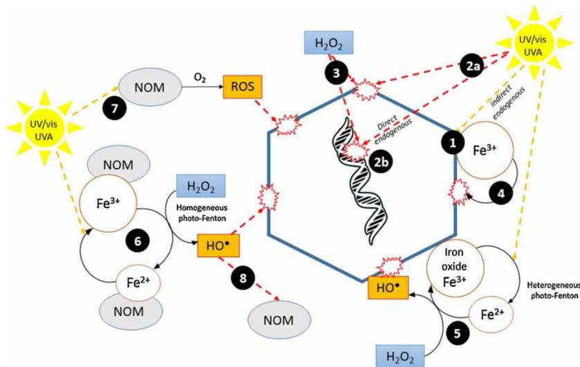
**Figure 4** | Mechanistic representation of possible pathways involved in the photo-inactivation of bacteriophage MS2 (Ortega-Gómez *et al.* 2015).
