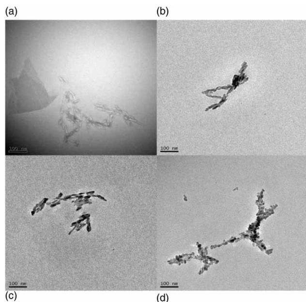
**Figure 1** | Transmission electron microscopy (TEM) micrograph: (a) activated carbon (GAC), (b) modified activated carbon – (GAC/NP1), (c) modified activated carbon – (GAC/NP4), and (d) modified activated carbon – (GAC/NP6) (Shimabuku *et al.* 2018).
