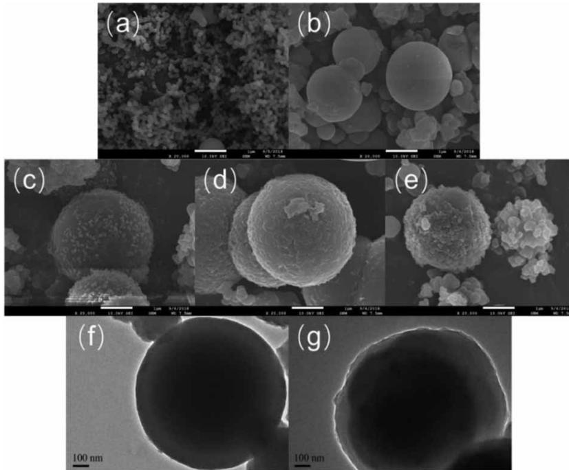
**Figure 2** | Scanning electron microscopy (SEM) images: (a) HTCC, (b) O-g-C<sub>3</sub>N<sub>4</sub>, (c) O-g-C<sub>3</sub>N<sub>4</sub>/HTCC-1, (d) O-g-C<sub>3</sub>N<sub>4</sub>/HTCC-2, and (e) O-g-C<sub>3</sub>N<sub>4</sub>/HTCC-3, and TEM images: (f) O-g-C<sub>3</sub>N<sub>4</sub> and (g) O-g-C<sub>3</sub>N<sub>4</sub>/HTCC-2 (Zhang *et al.* 2019).
