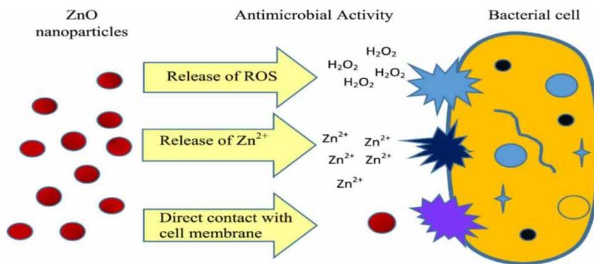
**Figure 3** | ZnO disinfection mechanisms (Dimapilis *et al.* 2018).
