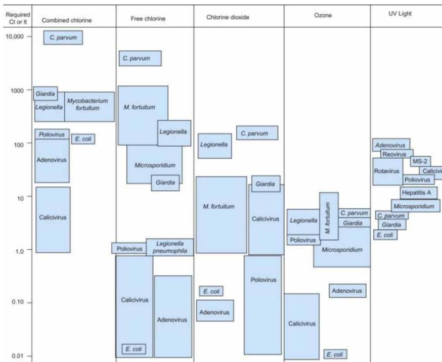
Figure 5 | Overview of disinfection requirements for 99% demobilization of microorganisms. Ct = concentration of disinfectant × time. It = (μW-s/cm<sup>2</sup>) (time) (Gerba 2015).
