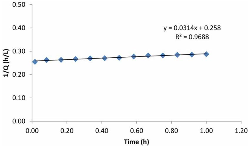
Figure 6 | Intermediate blocking model of PVDF membrane of applied pressure of 200 kPa.
