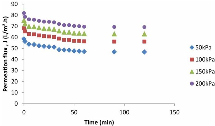
Figure 2 | Effect of applied pressures on permeate flux for PVDF membrane.
