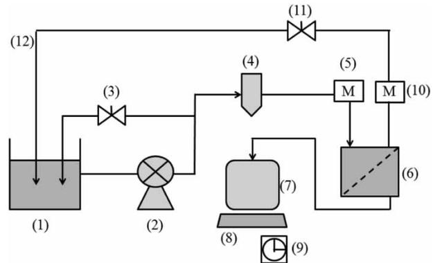
**Figure 1** | Schematic diagram of experimental setup. (1) Feed tank, (2) gear pump, (3) valve, (4) flow rate indicator, (5) manometer, (6) UF membranes module, (7) permeate tank, (8) electronic balance, (9) stop watch, (10) manometer, (11) valve, and (12) return of concentrate stream.
