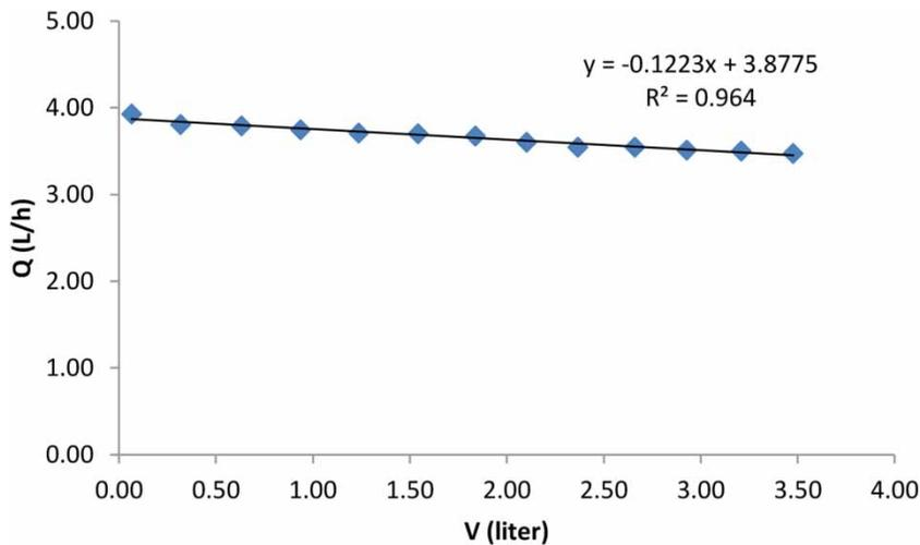
Figure 7 | Complete blocking model of PVDF membrane of applied pressure of 200 kPa.
