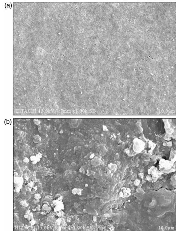
Figure 8 | SEM image of PVDF membrane: (a) new membrane; (b) fouled membrane.
