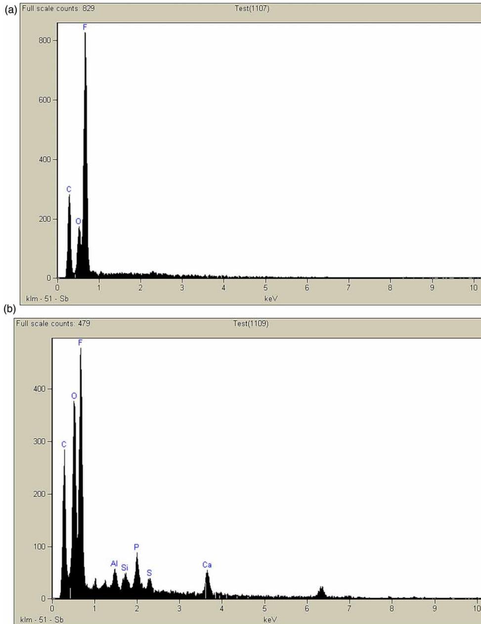
**Figure 10** | EDX analysis of PVDF membrane: (a) new membrane; (b) fouled membrane.
