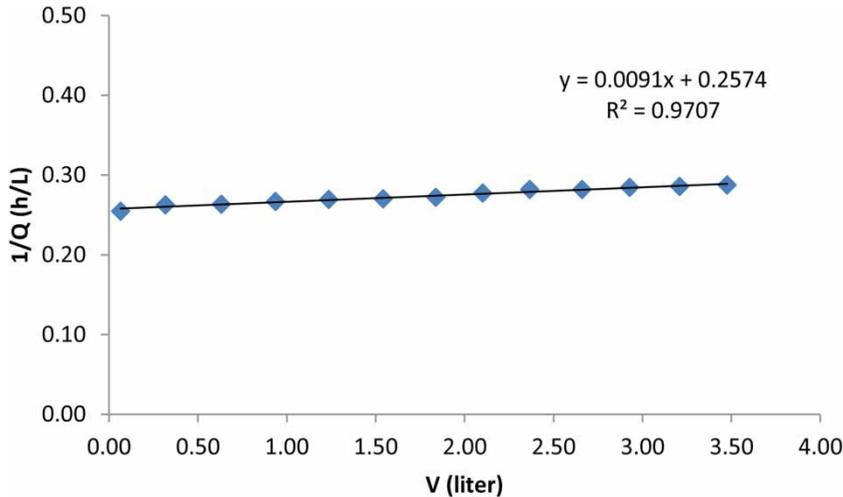
**Figure 4** | Cake filtration model of PVDF membrane of applied pressure of 200 kPa.
