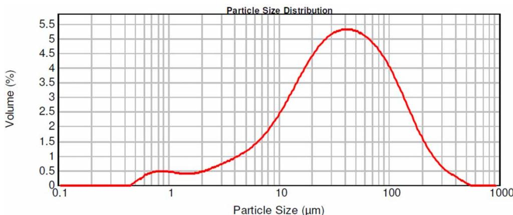
Figure 9 | Particle size distribution of foulant on PVDF membrane.
