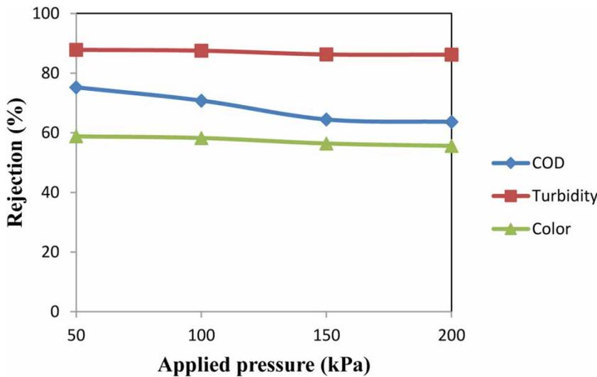
Figure 3 | Effect of applied pressure on percentage rejection of pollutants of PVDF membrane.
