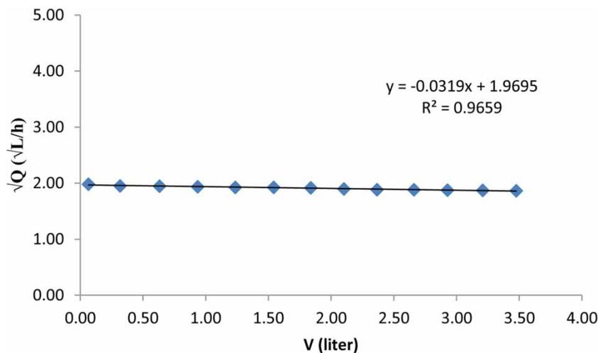
**Figure 5** | Standard blocking model of PVDF membrane of applied pressure of 200 kPa.
