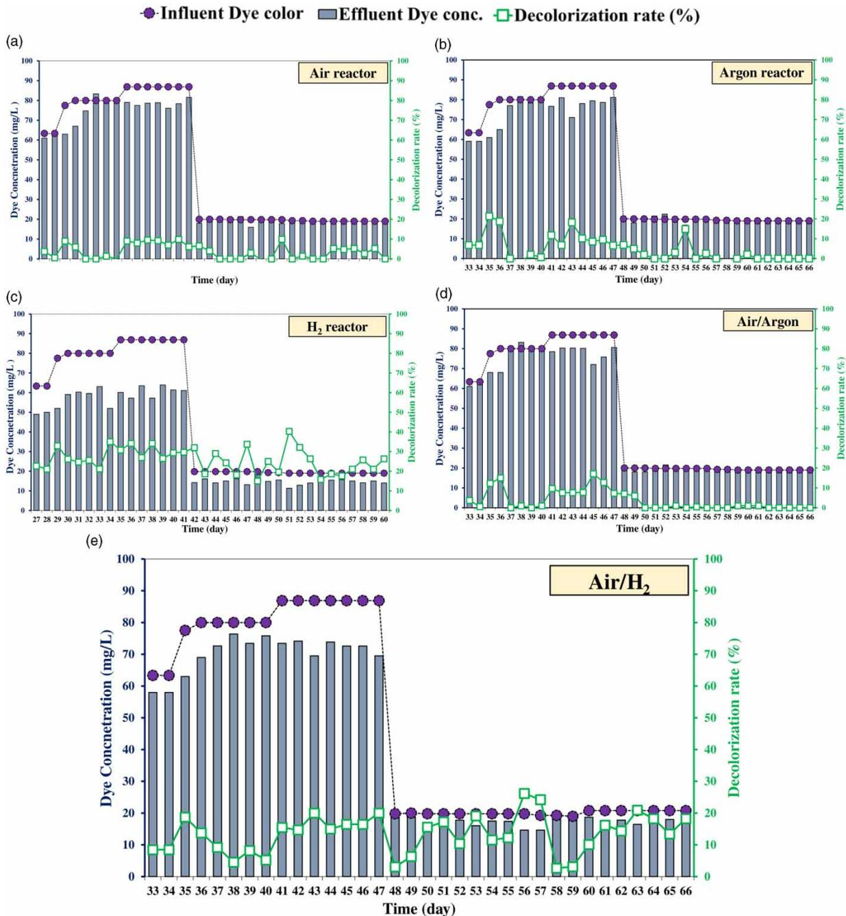
**Figure 3** | RB-5 dye concentrations and decolorization rate. (a) from Air reactor; (b) Argon reactor; (c) H<sub>2</sub> reactor; (d) Air/argon reactor; (e) Air/H<sub>2</sub> reactor.
