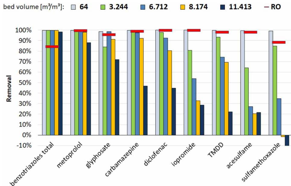
**Figure 3** | Retention of micropollutants in the GAC filter according to treated bed volumes ( $\text{m}^3$  filtrate/ $\text{m}^3$  GAC filter bed) and the averaged retention by the RO membrane over the entire operation time.
