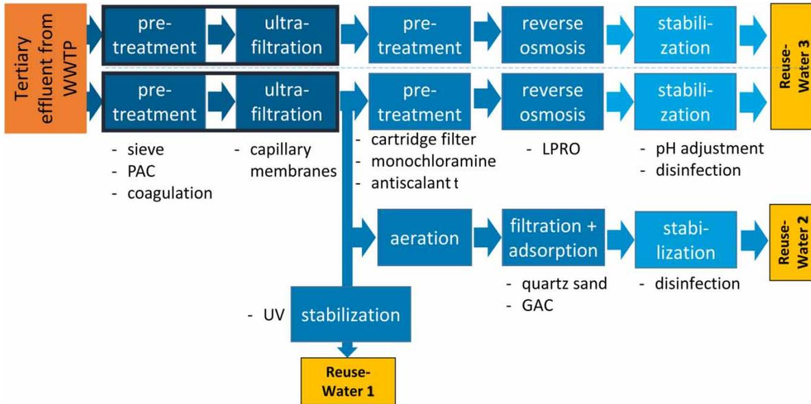
Figure 1 | Flow chart of the pilot plant.
