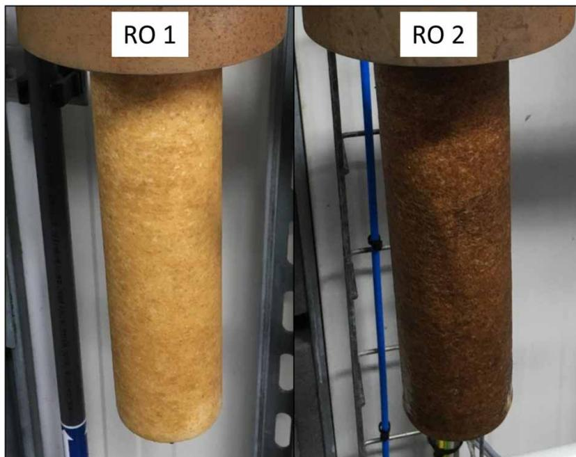
Figure 7 | Cartridge filters of RO1 (with NH<sub>2</sub>Cl) and RO2 (without NH<sub>2</sub>Cl) in comparison after 4 weeks of operation (26 June 2019–23 July 2019).
