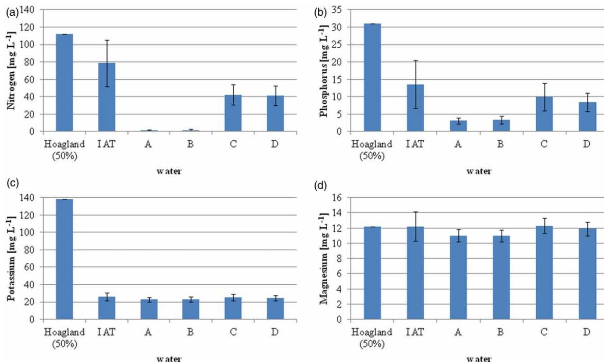
**Figure 2** | Average concentrations of N, P, K and Mg in the inflow of the aeration tank (IAT) and the effluent of the differently treated wastewaters (a, b, c and d) in comparison to the reference nutrient solution (2017–2018).
