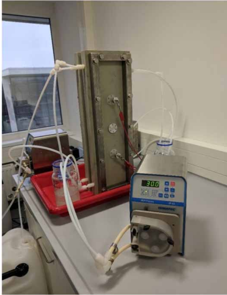
Figure 6 | The ED system used for treatment of the membrane permeates out of the pilot in the ceramic industry (source: Friedrich, IKTS).
