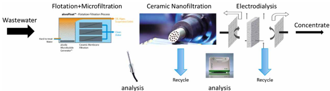
Figure 1 | The integrated process steps being inspected in the PAKmem project (sources: Fraunhofer IKTS, akvola, LUM, SOPAT).
