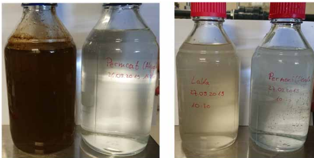
Figure 7 | Samples taken from the feed to the plant (left bottles, produced water after primary treatment) and post flotation-MF (right bottles, always clear water). The two images were taken on two consecutive days.
