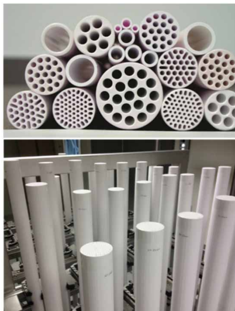
Figure 3 | Ceramic tubular NF membranes used in the pilots (source: IKTS, Rauschert).
