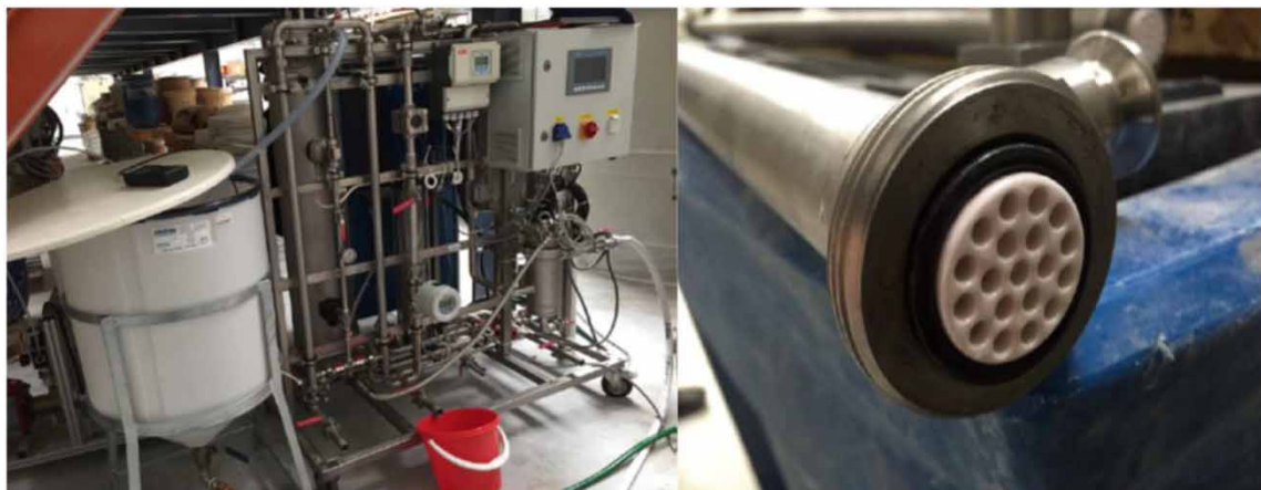
Figure 5 | NF pilot plant used in the ceramics industry.
