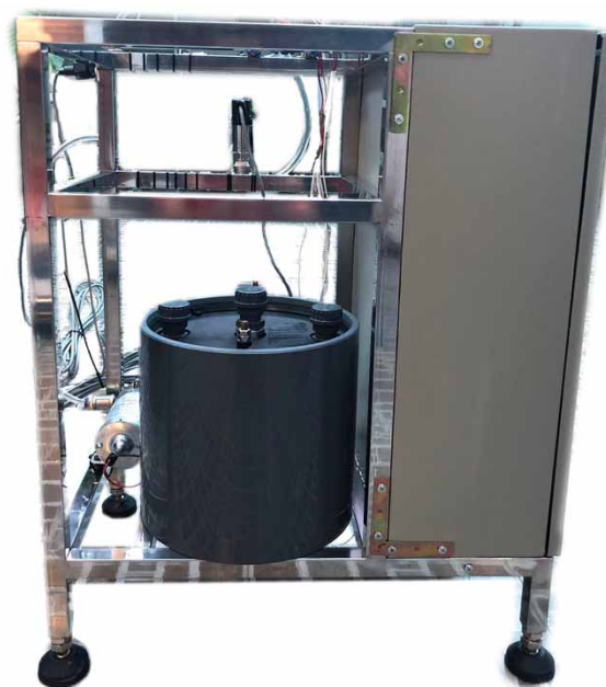
Figure 2 | MCDI pilot plant for desalination including the electrode module (Voltea C3) and power supply (XP Power HDS 1500 PS12).
