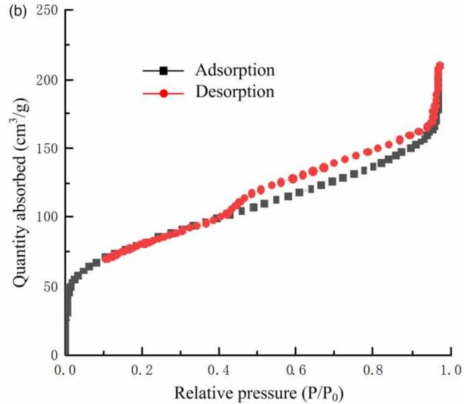
**Figure 1** |  $N_2$  adsorption-desorption isotherms of SAC and MSAC.
