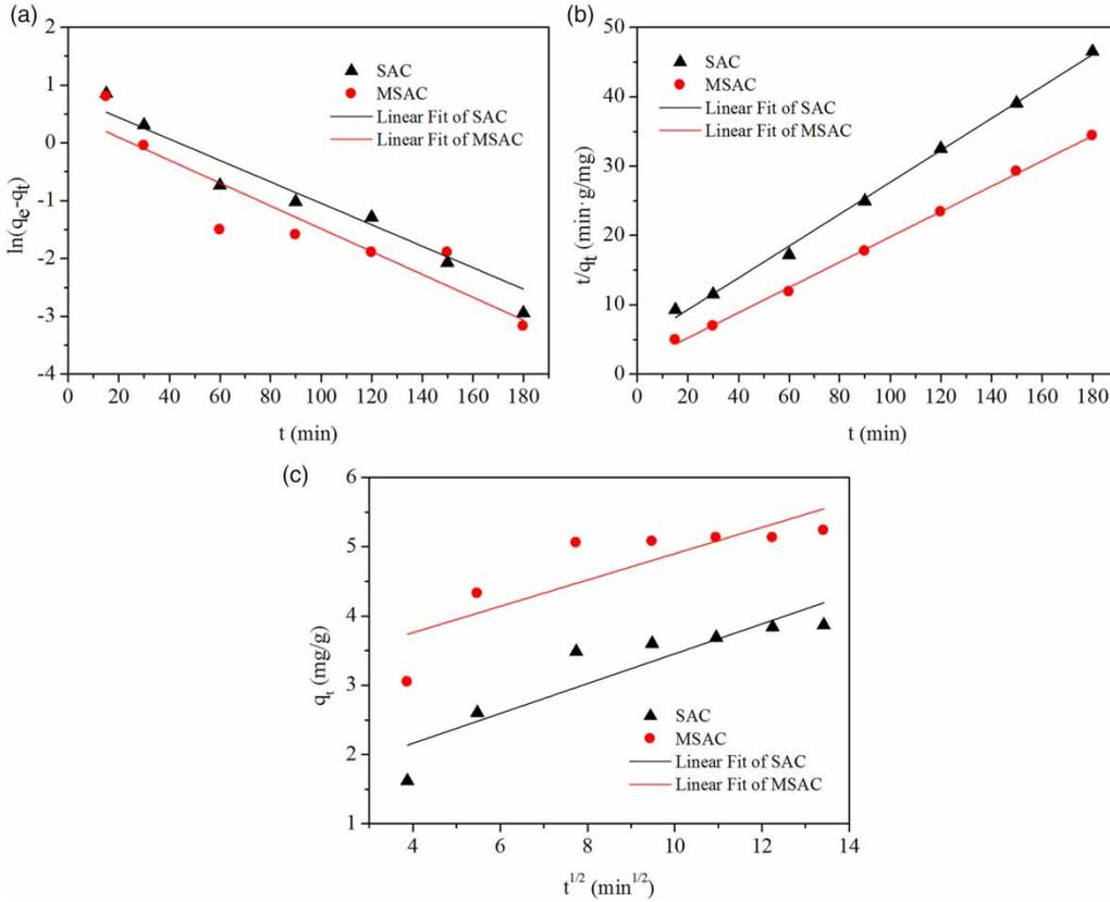
**Figure 5** | Adsorption kinetics of AMX removal by SAC and MSAC: (a) PFO model, (b) PSO model and (c) IPD model.
