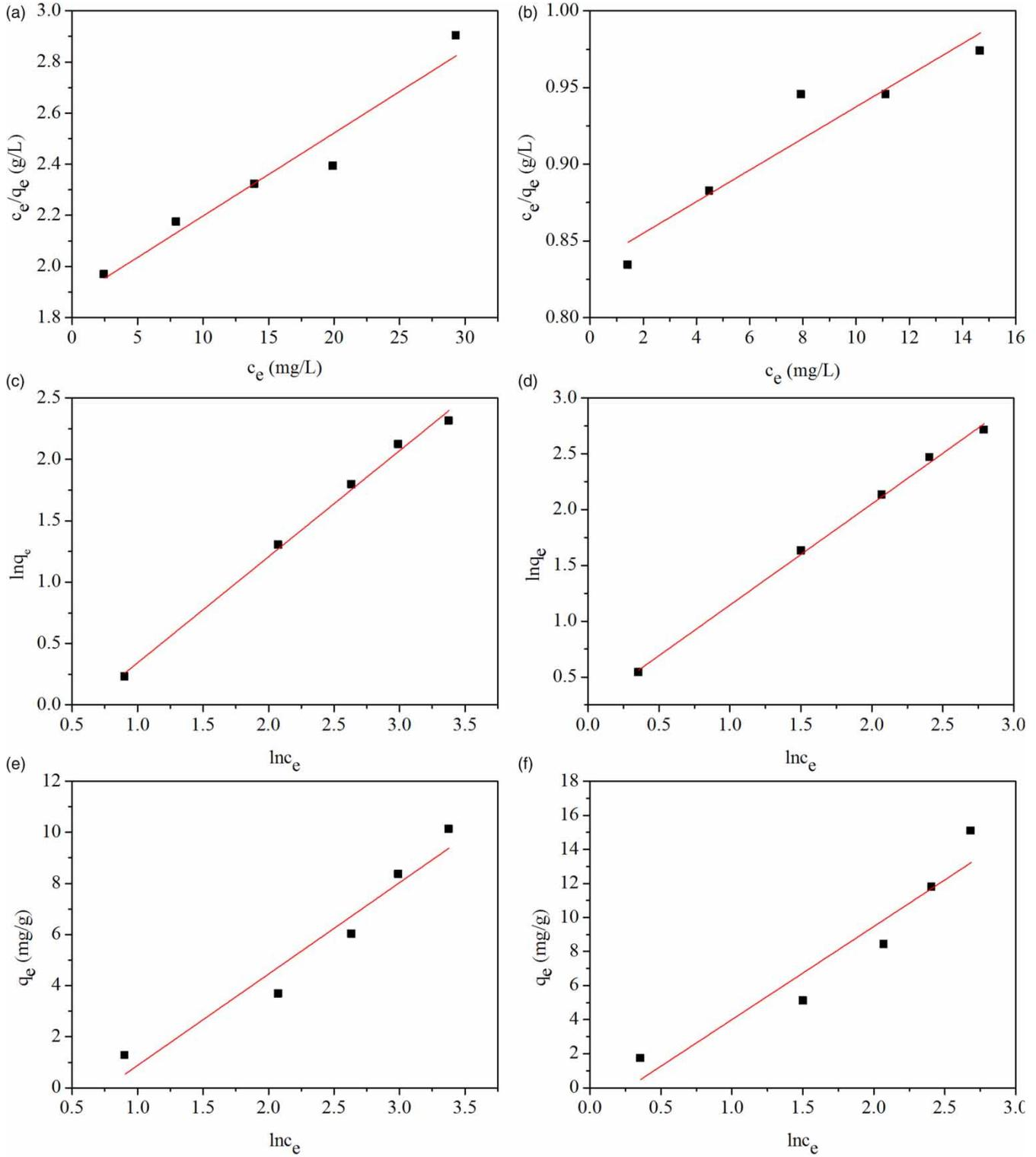
**Figure 6** | (a) Langmuir isotherm, (c) Freundlich isotherm, (e) Temkin isotherm models of AMX onto SAC, and (b) Langmuir isotherm, (d) Freundlich isotherm, (f) Temkin isotherm models of AMX onto MSAC.
