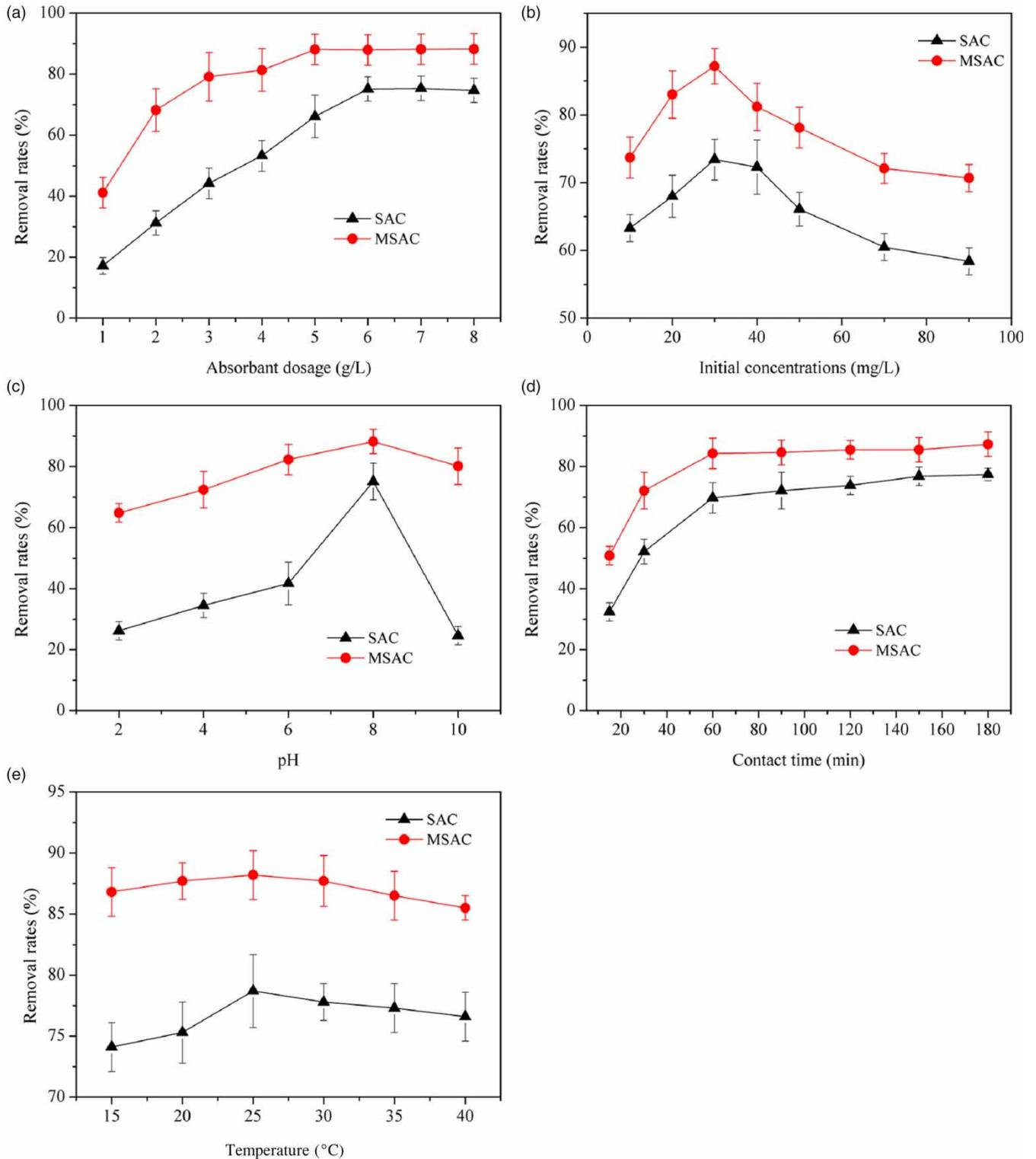
**Figure 4** | Effect of: (a) AC dosages, (b) initial concentrations, (c) pH, (d) contact time, and (e) temperature on adsorption of AMX onto MSAC. Error bars represent the range of data from duplicate experiments.
