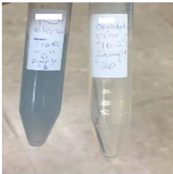
**Figure 10** | Discoloration of textile wastewater after 6 hours of electrolysis with BDD anode using  $\text{NaCl}$  as supporting electrolyte ( $2.8 \text{ mA/cm}^2$ ,  $25^\circ\text{C}$ ,  $1 \text{ g/L Na}_2\text{SO}_4$ ,  $1 \text{ g/L NaCl}$ ,  $\text{pH} = 5.4$ ).
