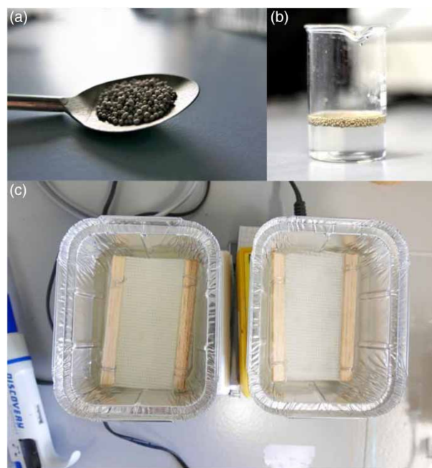
Figure 4 | (a) Glass foam, (b) floating glass foam, and (c) glass fiber with floaters.
