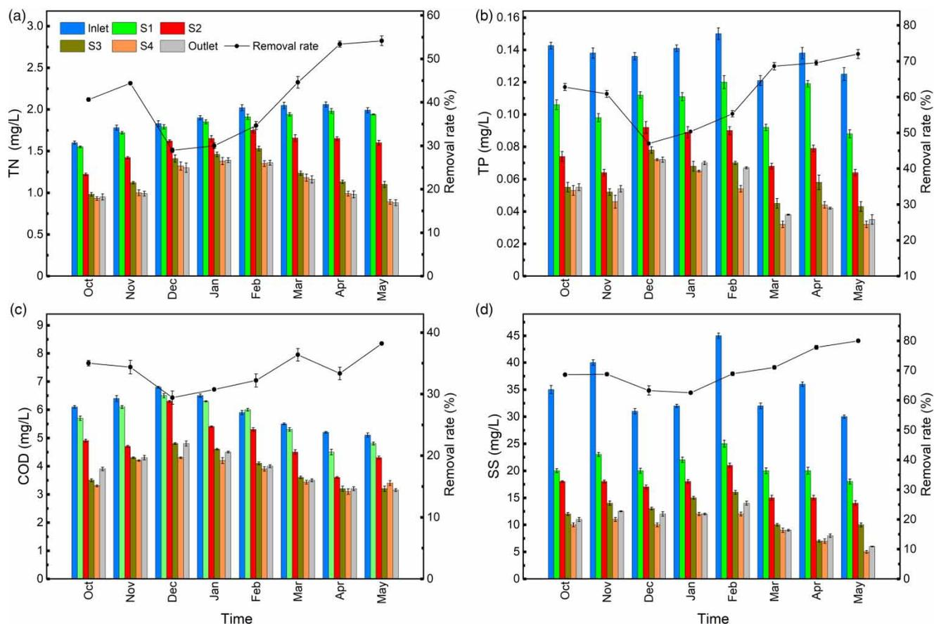
**Figure 3** | Variations and removal rates of TN (a), TP (b), COD (c) and SS (d) for the system.
