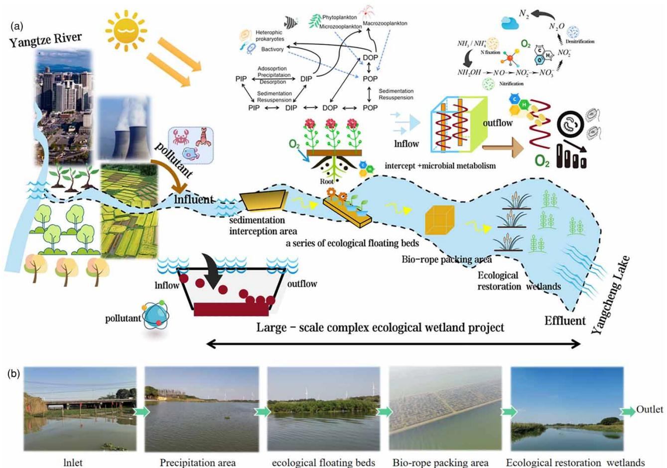
**Figure 2** | The process of composite ecological engineering (a) and site photographs (b).
