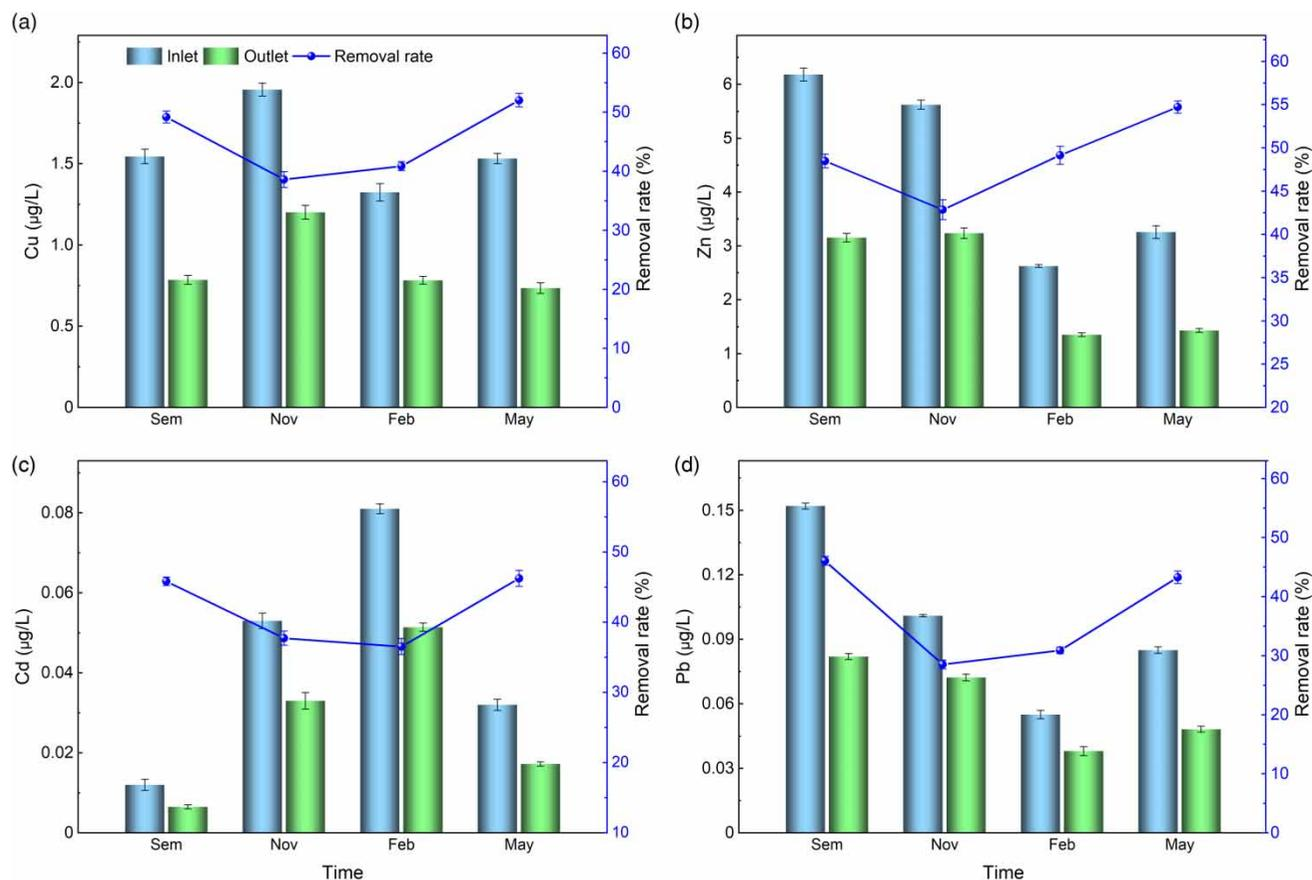
**Figure 4** | Variations and removal rates of Cu (a), Zn (b), Cd (c) and Pb (d) for the system.
