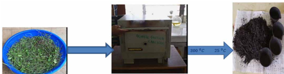
Figure 2 | Khat waste pyrolysis processes during biochar production.
