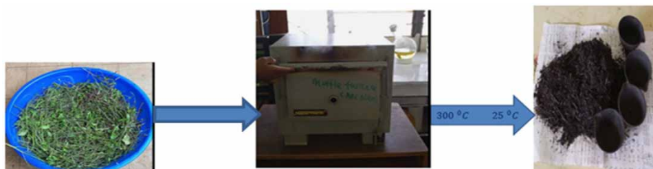
Figure 2 | Khat waste pyrolysis processes during biochar production.
