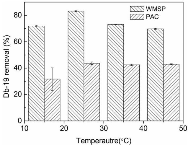
**Figure 6** | Effect of temperature on DB-19 removal ( $C_0 = 30$  mg/L, pH = 8, settling time = 120 min).
