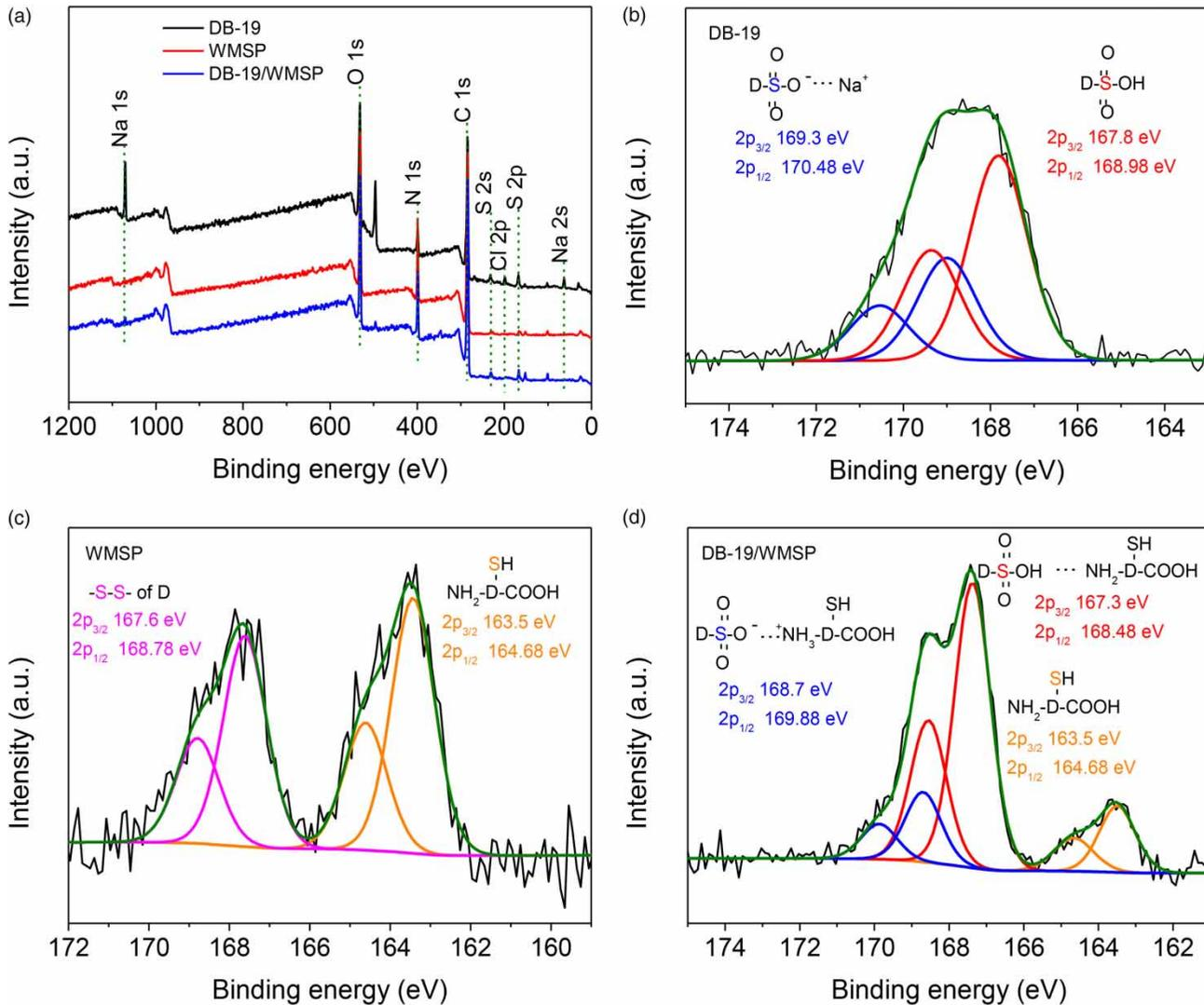
**Figure 10** | XPS survey spectra of wide scan of DB-19, WMSP and DB-19/WMSP floes (a); high magnification of S 2p of DB-19 (b); high magnification of S 2p of WMSP (c); high magnification of S 2p of DB-19/WMSP floes (d), where D and W represent DB-19 and WMSP, respectively.
