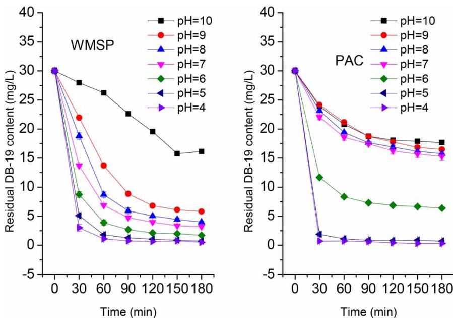
Figure 3 | Effect of settling time on DB-19 removal ( $C_0 = 30 \text{ mg/L}$ ,  $T = 25^\circ \text{C}$ , WMSP and PAC dosage:  $5.29 \text{ mg/L}$ ).
