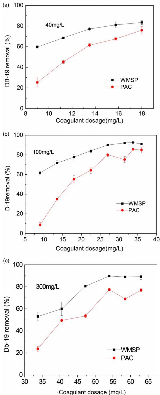
**Figure 5** | Effect of coagulant dosage on DB-19 removal (pH = 8,  $T = 25$  °C, settling time = 120 min).
