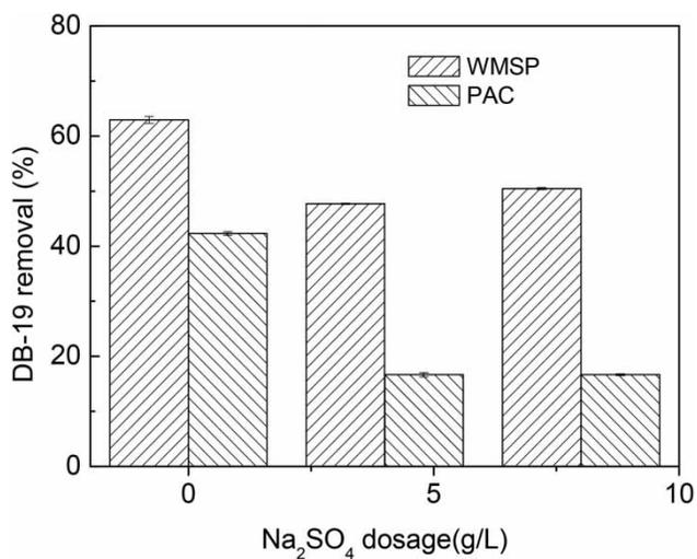
**Figure 7** | Effect of inorganic salt on DB-19 removal by WMSP and PAC on DB-19 removal ( $C_0 = 30$  mg/L, pH = 8, settling time = 2 h).
