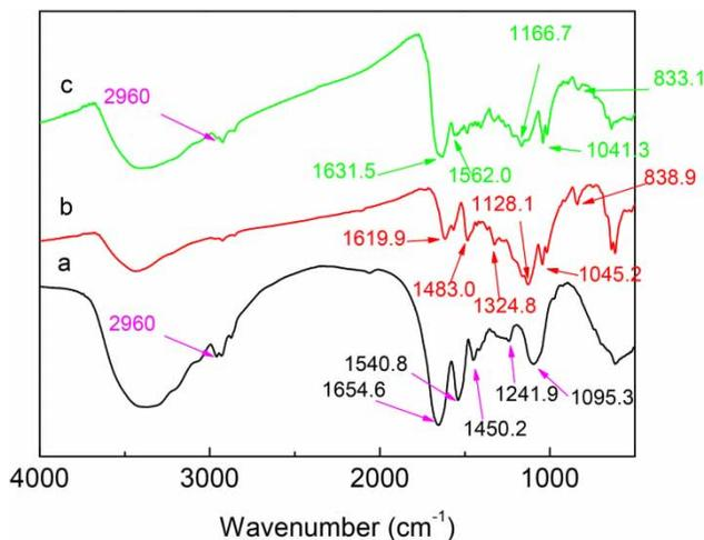
**Figure 9** | FTIR of WMSP (a), DB-19 (b), DB-19/WMSP flocs (c).
