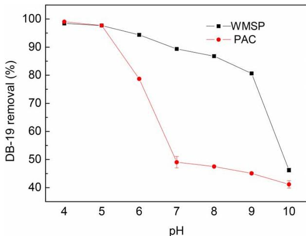
**Figure 4** | Effect of pH on DB-19 removal ( $C_0 = 30$  mg/L,  $T = 25$  °C, time = 180 min).
