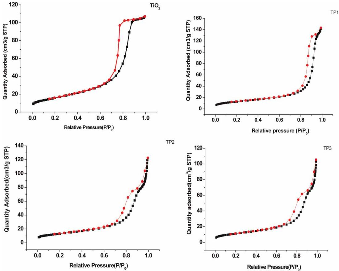
**Figure 3** |  $N_2$  adsorption-desorption isotherms and pore diameter distributions of pure and polyaniline modified  $TiO_2$  samples.
