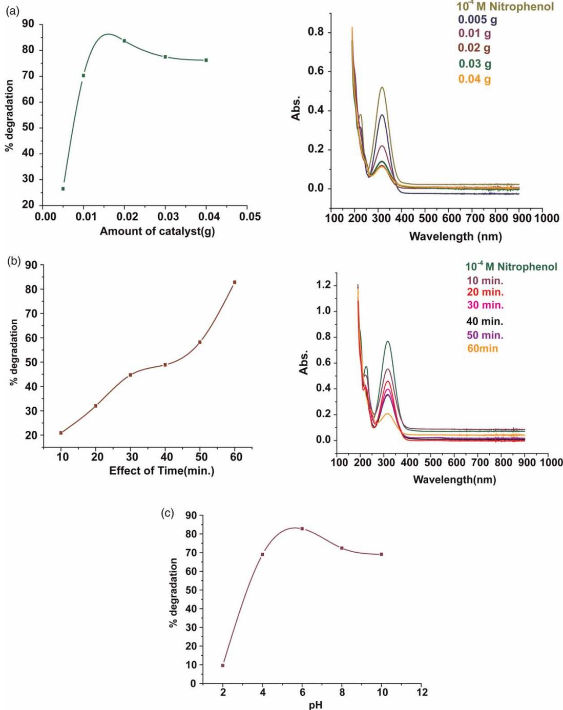
**Figure 9** | (a) Effect of amount of catalyst. (b) Effect of time on photocatalytic degradation of 4-NP. (c) Effect of pH on degradation of nitrophenol. (d) Variation of absorption maxima of 4-NP in acidic and basic pH. (e) Effect of polyaniline content. (f) Recyclability study. (continued)
