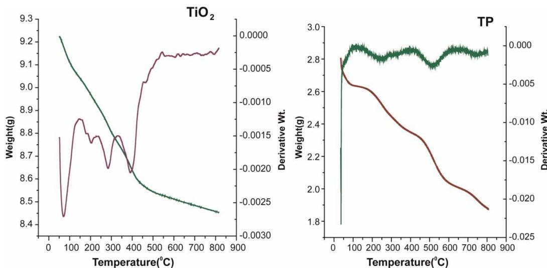
Figure 6 | TG-DTG pattern of pure  $\text{TiO}_2$  and polyaniline modified  $\text{TiO}_2$  (TP).
