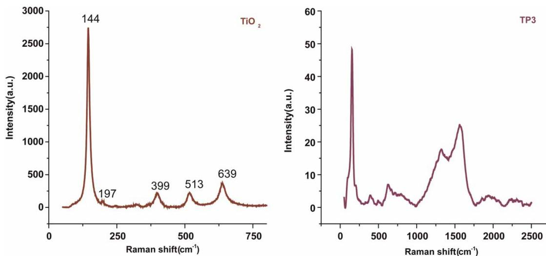
Figure 5 | Raman spectra of pure TiO<sub>2</sub> and polyaniline modified TiO<sub>2</sub> (TP).
