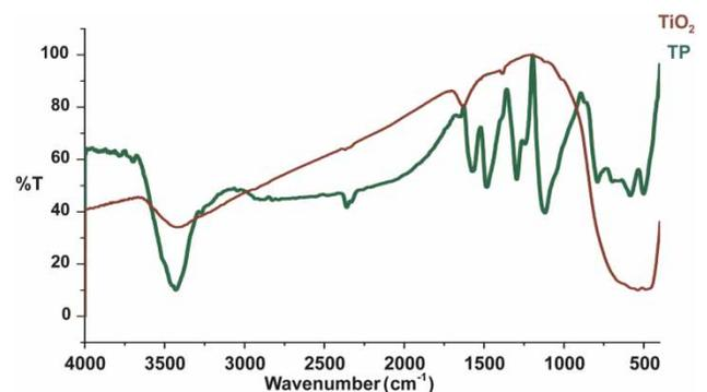
**Figure 4** | FTIR spectra of pure  $TiO_2$  and polyaniline modified  $TiO_2$  (TP).
