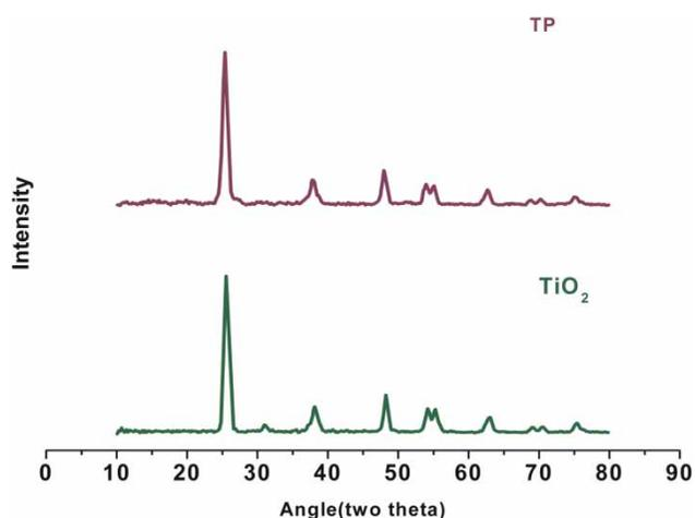
Figure 1 | XRD Pattern of pure TiO<sub>2</sub> and polyaniline modified TiO<sub>2</sub> (TP).
