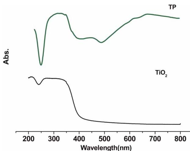
Figure 2 | UV-VIS DRS spectra of pure TiO<sub>2</sub> and polyaniline modified TiO<sub>2</sub> (TP).
