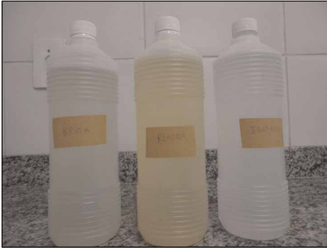
Figure 2 | Samples of raw water, pretreated water by the reactor and treated water (left to right).
