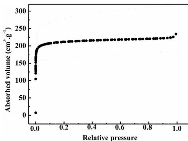
Figure 3 | Cryogenic N<sub>2</sub> adsorption–desorption isotherm of NPR.
