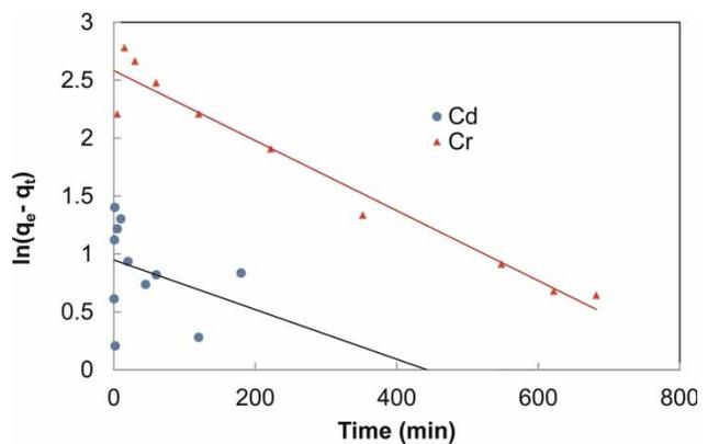
Figure 8 | Pseudo-first-order kinetic plots for Cr(VI) and Cd(II) adsorption onto NPR.
