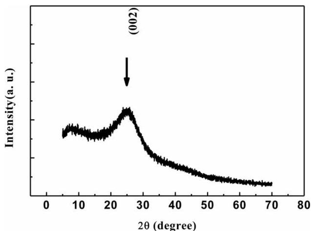
Figure 2 | XRD patterns of NPR.
