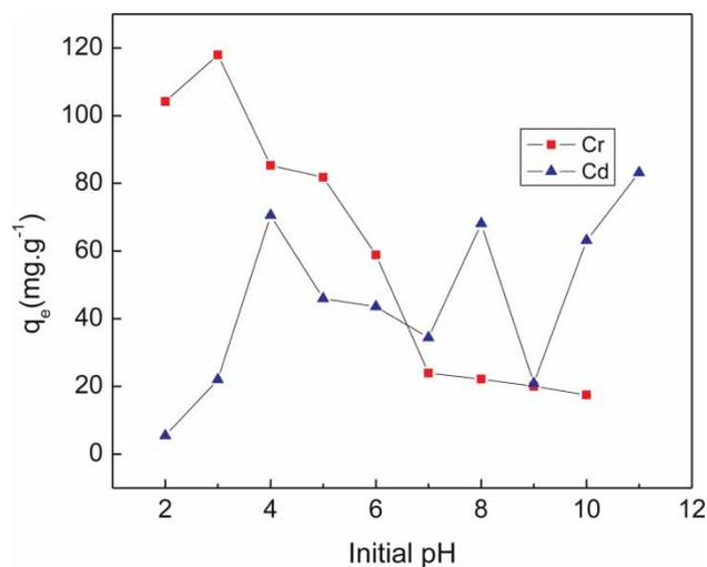
Figure 6 | Effect of initial pH on the removal of Cd(II) and Cr(VI) using NPR.
