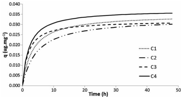
**Figure 3** | Pseudo-second-order kinetic non-linear curves for adsorption of dc-STX on C1, C2, C3 and C4 coconut shell GAC samples.
