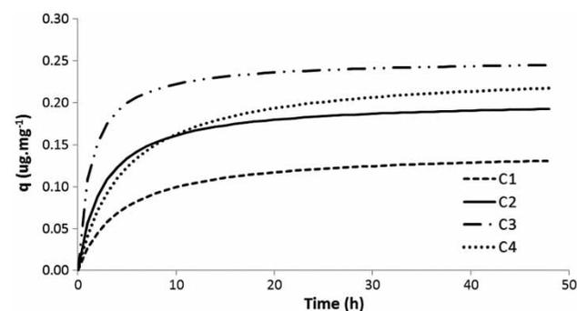
**Figure 2** | Pseudo-second-order kinetic non-linear curves for adsorption of STX on C1, C2, C3 and C4 coconut shell GAC samples.
