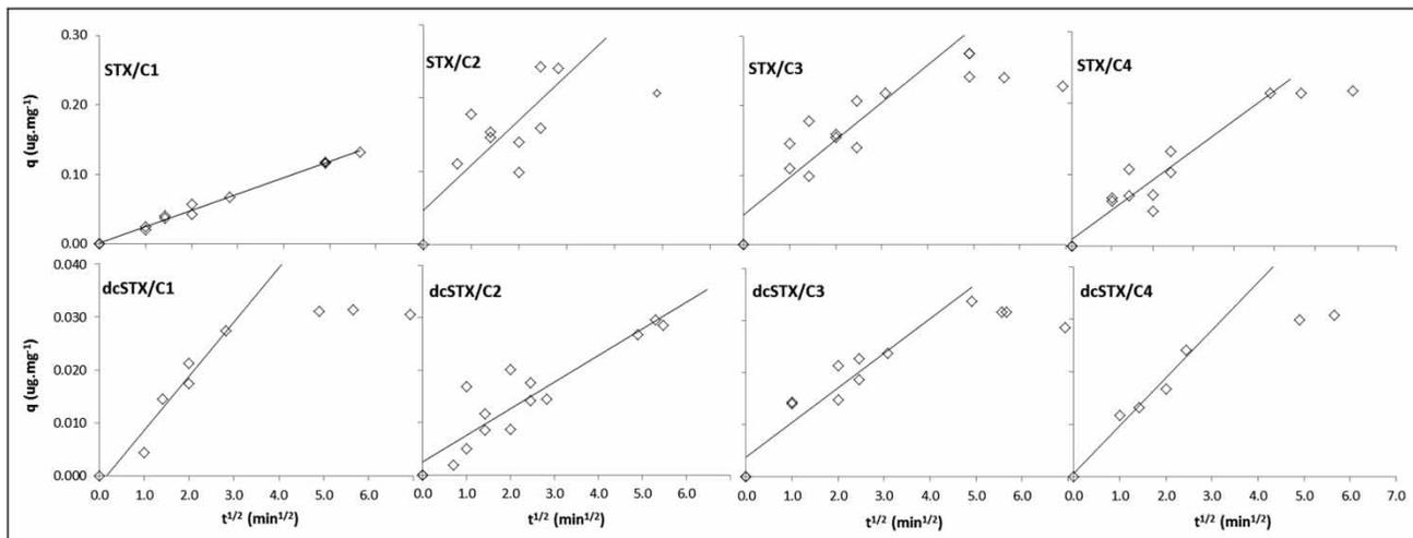
**Figure 4** | Intraparticle diffusion model for adsorption of STX and dc-STX on GAC samples C1, C2, C3 and C4.
