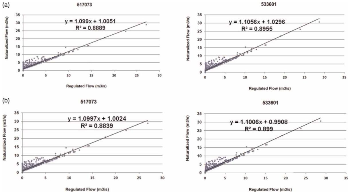
Figure 4 | Regression equation for monthly naturalized and regulated flow with full authorization and current use data. (a) Full authorization; (b) current use.
