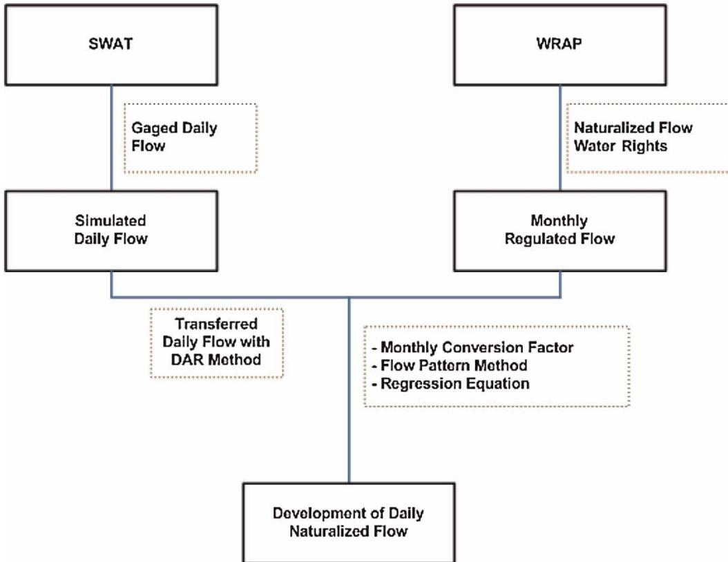
**Figure 2** | Flow chart for disaggregating monthly flows.
