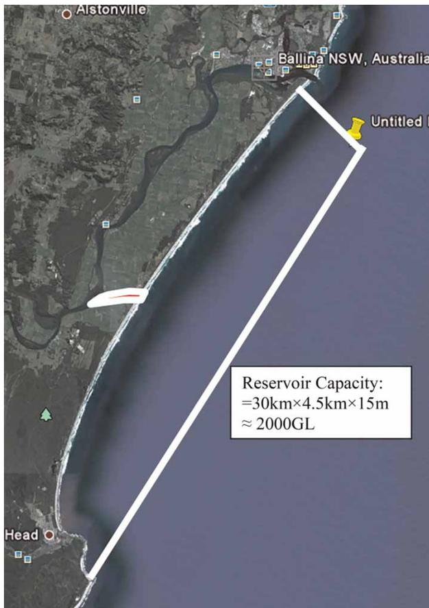
**Figure 5** | Proposed coastal reservoir for Richmond River, solid lines are the dam wall and canal that divert the stormwater to the coastal reservoir (solid lines are proposed works).
