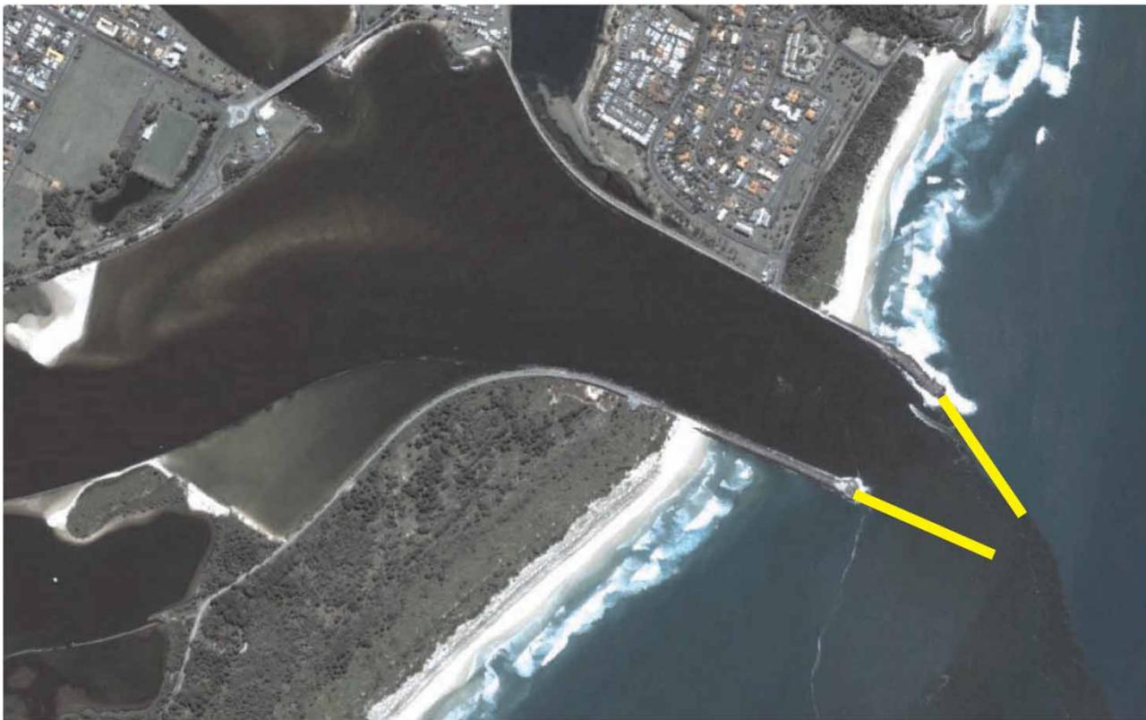
**Figure 6** | To reduce seawater pollution in the river, the existing seawalls at Ballina at the mouth of the River Richmond are suggested to be extended into the sea (solid lines are proposed works).
