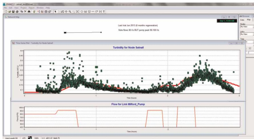
**Figure 13** | Six month regeneration trial PODDS EPANET modelling results (upper plot shows turbidity with squares measured data, and continuous line modelled result; the lower plot shows model flow demand).
