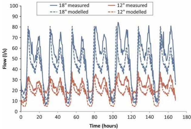
**Figure 4** | Measured and modelled flows, 18" (higher flow) and 12" trunk mains.
