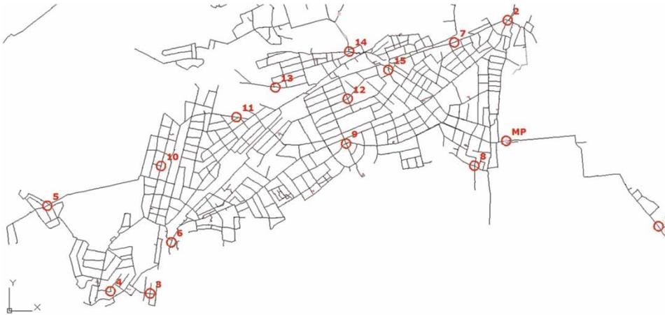
**Figure 8** | Pressure measurement points for Zone 11.
