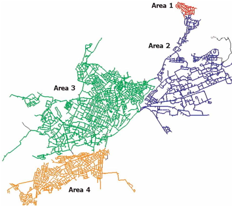
**Figure 9** | Four main network areas that can be run separately.
