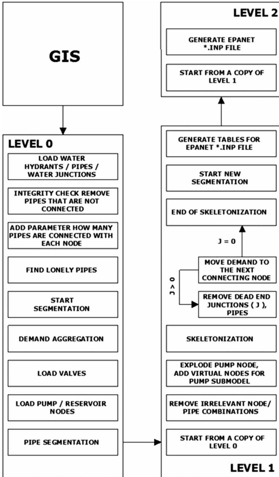
Figure 2 | Main simplification procedures at SQL-based database level.
