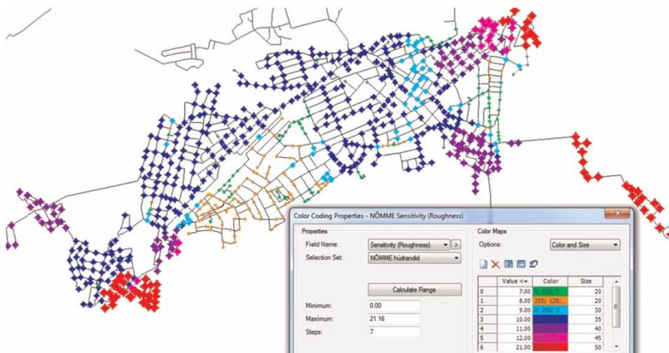
Figure 6 | Roughness sensitivity map for Zone 11. Larger node sizes indicates more sensitivity.
