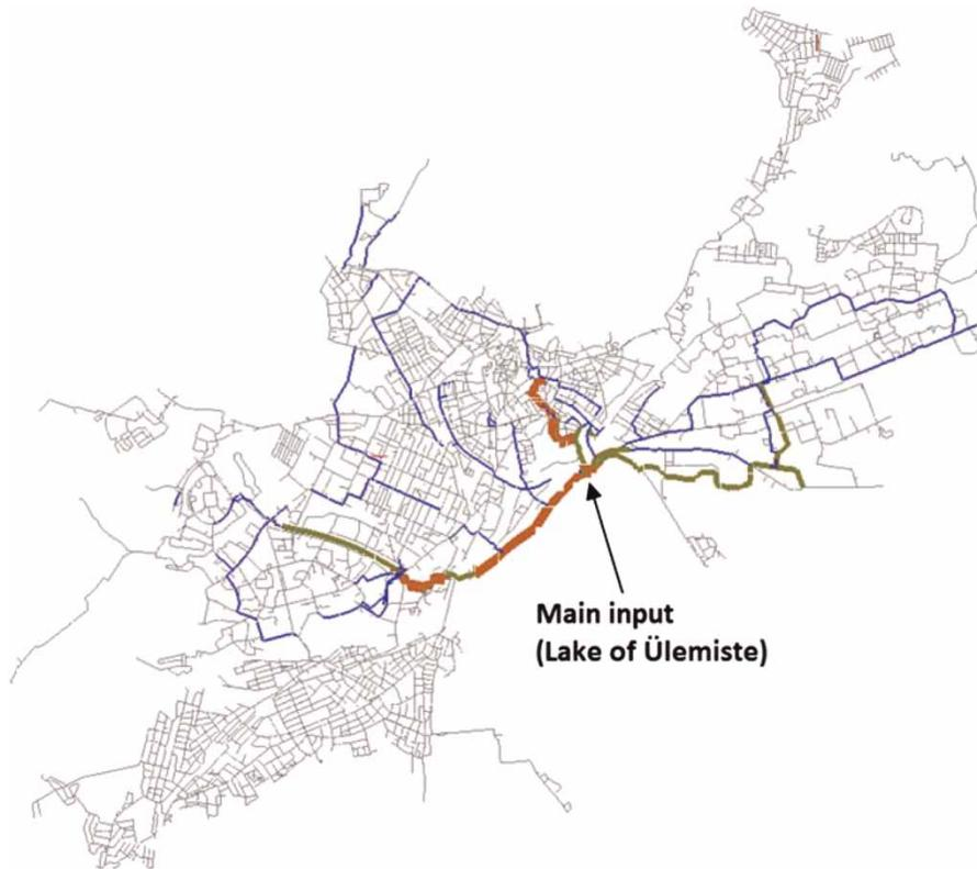
**Figure 1** | Hydraulic water network model with highlighted transmission lines.
