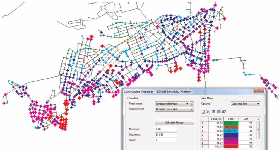
**Figure 7** | Fire flow sensitivity map for Zone 11. Larger node sizes indicates more sensitivity.
