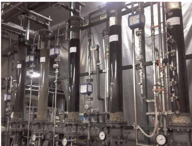
Figure 2 | Fixed bed filter pilot plant.
