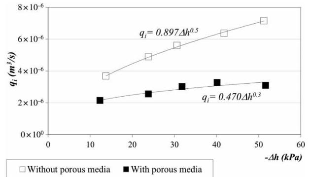
Figure 10 | Orifice equation with porous media for round hole of 1 mm.
