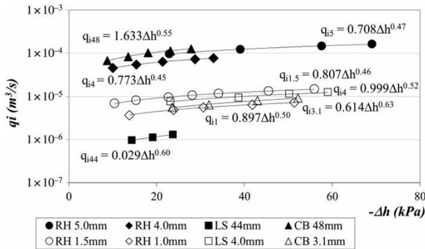
Figure 8 | Equation (5) for diverse failures.
