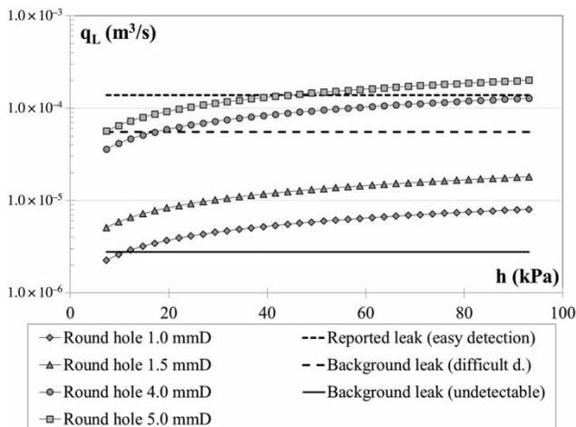
Figure 2 | Leakage flows through different round holes in a range 0–98.1 kPa.
