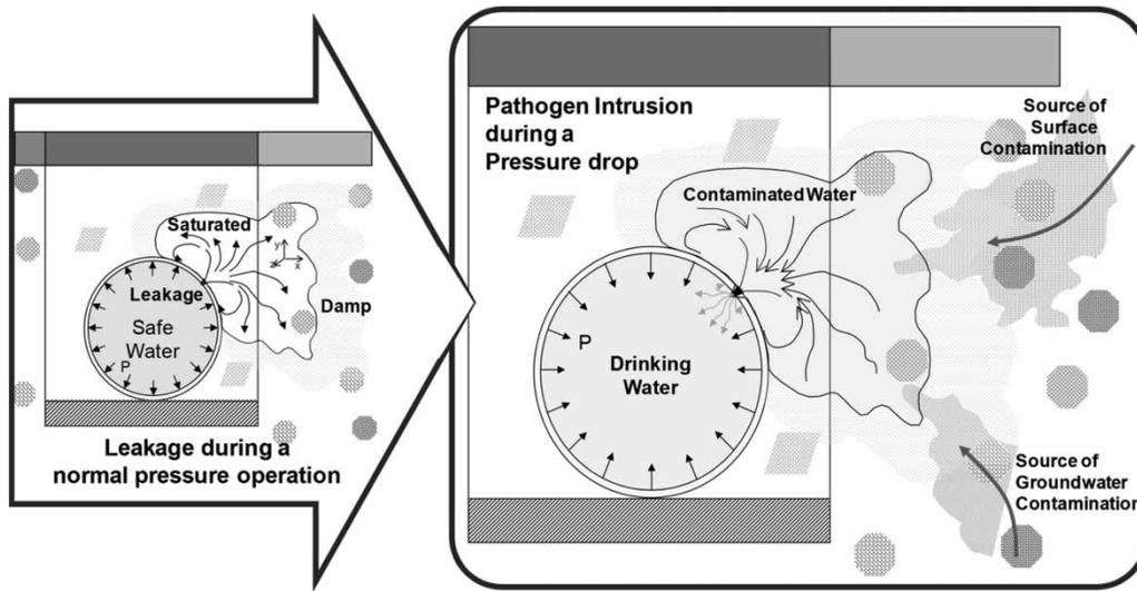
Figure 1 | Pathogen intrusion through a failure in pipes.
