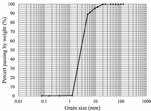
**Figure 6** | Granulometric composition of the fine gravel.
