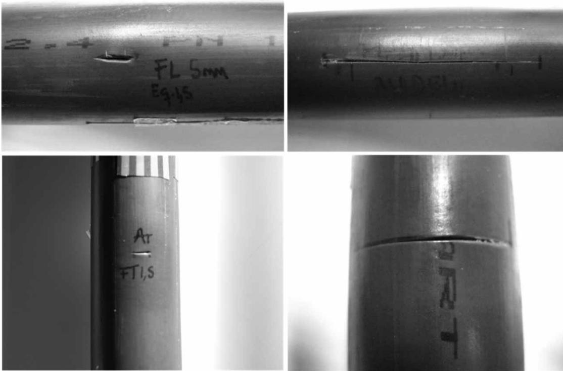
**Figure 3** | Longitudinal splits and circumferential breaks.
