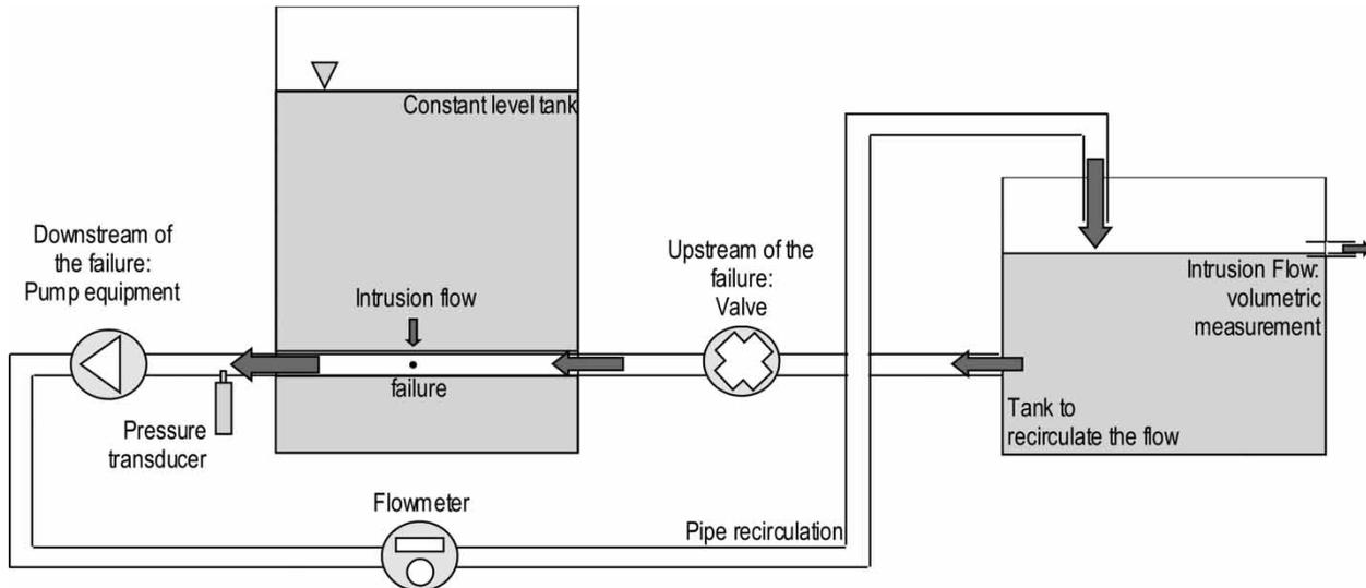
Figure 5 | Schema of the physical intrusion flow model.
