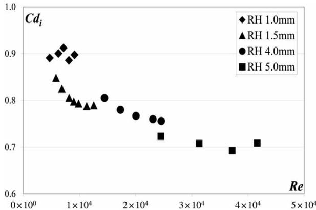
Figure 11 |  $C_{di}$  for round hole failures.
