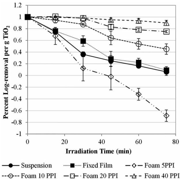
Figure 9 | Log-removal of *E. coli* per g of  $\text{TiO}_2$ .
