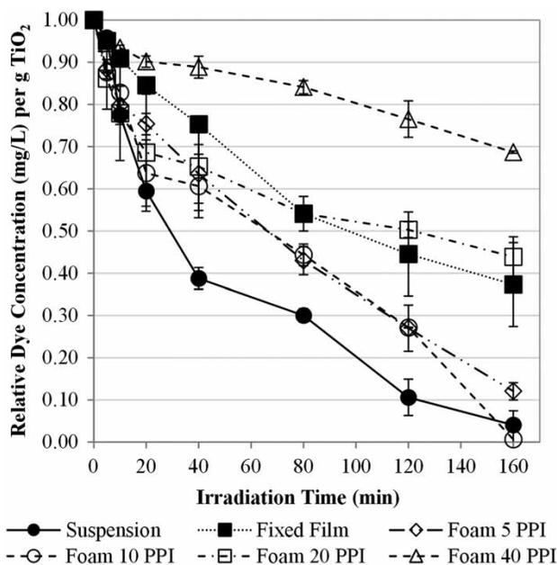
**Figure 5** | Relative loss of MB for  $\text{TiO}_2$ -containing suspension, fixed film and foams of 5, 10, 20 and 40 PPI.
