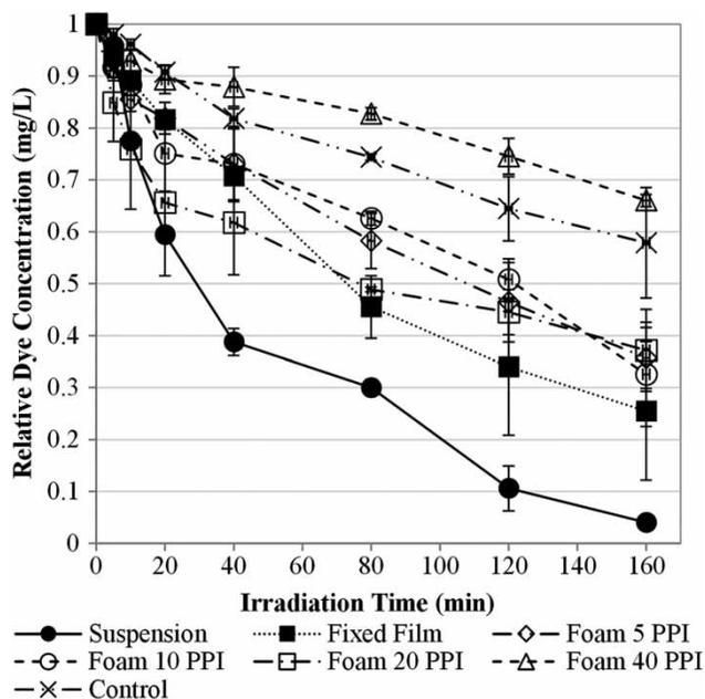
**Figure 4** | Relative loss of MB for  $\text{TiO}_2$ -containing suspension, fixed film and foams of 5, 10, 20 and 40 PPI.
