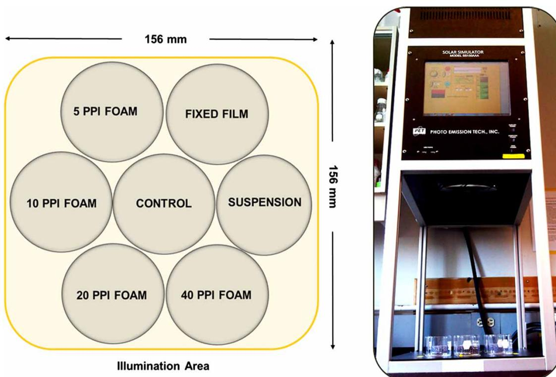
**Figure 2** | Left – reactors arranged in solar simulator during treatment; right – photoemission Tech SS150AA solar simulator.
