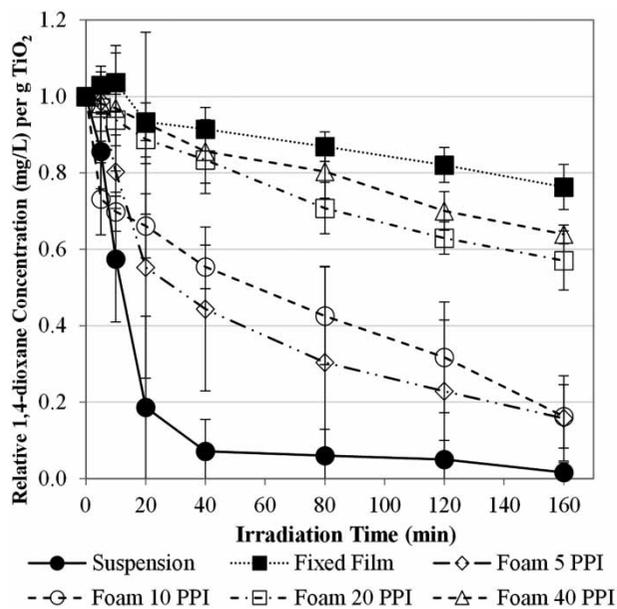
Figure 7 | Relative loss of 1,4-dioxane per g of TiO<sub>2</sub>.
