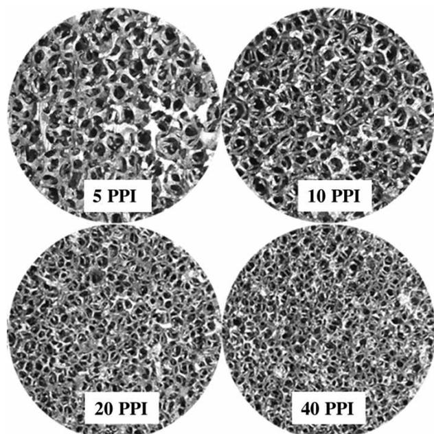
Figure 1 | Aluminum foams with 5, 10, 20 and 40 PPI.
