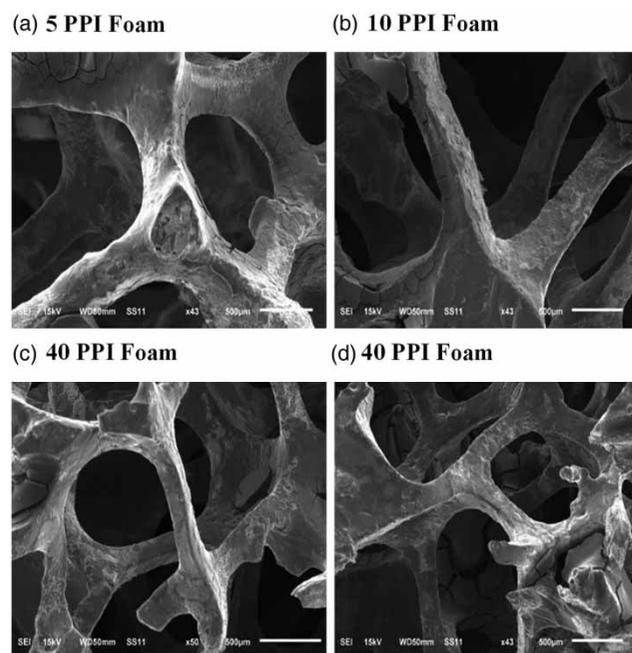
**Figure 3** | SEM secondary electron images (SEI) of TiO<sub>2</sub> coated aluminum foams.
