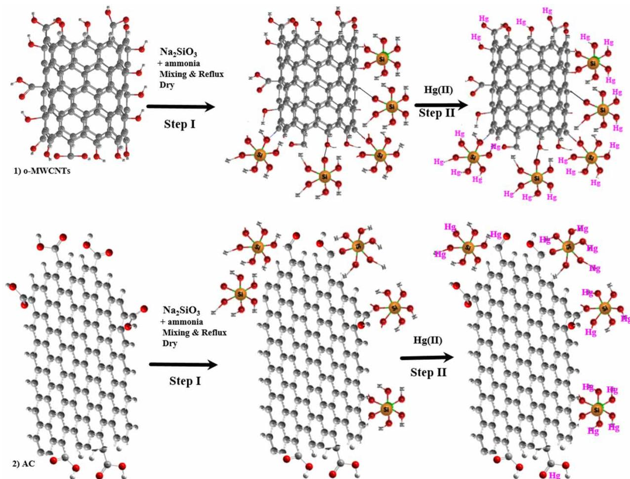
Figure 1 | Schematic illustration of silica /CNT and silica/AC preparation.
