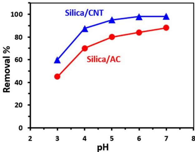
**Figure 7** | Effect of pH on the adsorption of Hg<sup>2+</sup> ions on silica/CNT and silica/AC.
