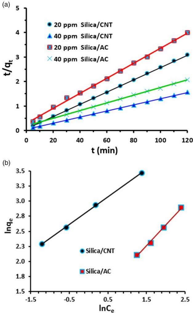
**Figure 8** | Pseudo-second order kinetic plot (a) and Freundlich adsorption isotherm (b) for  $\text{Hg}^{2+}$  adsorption on Silica/CNT and Silica/AC.
