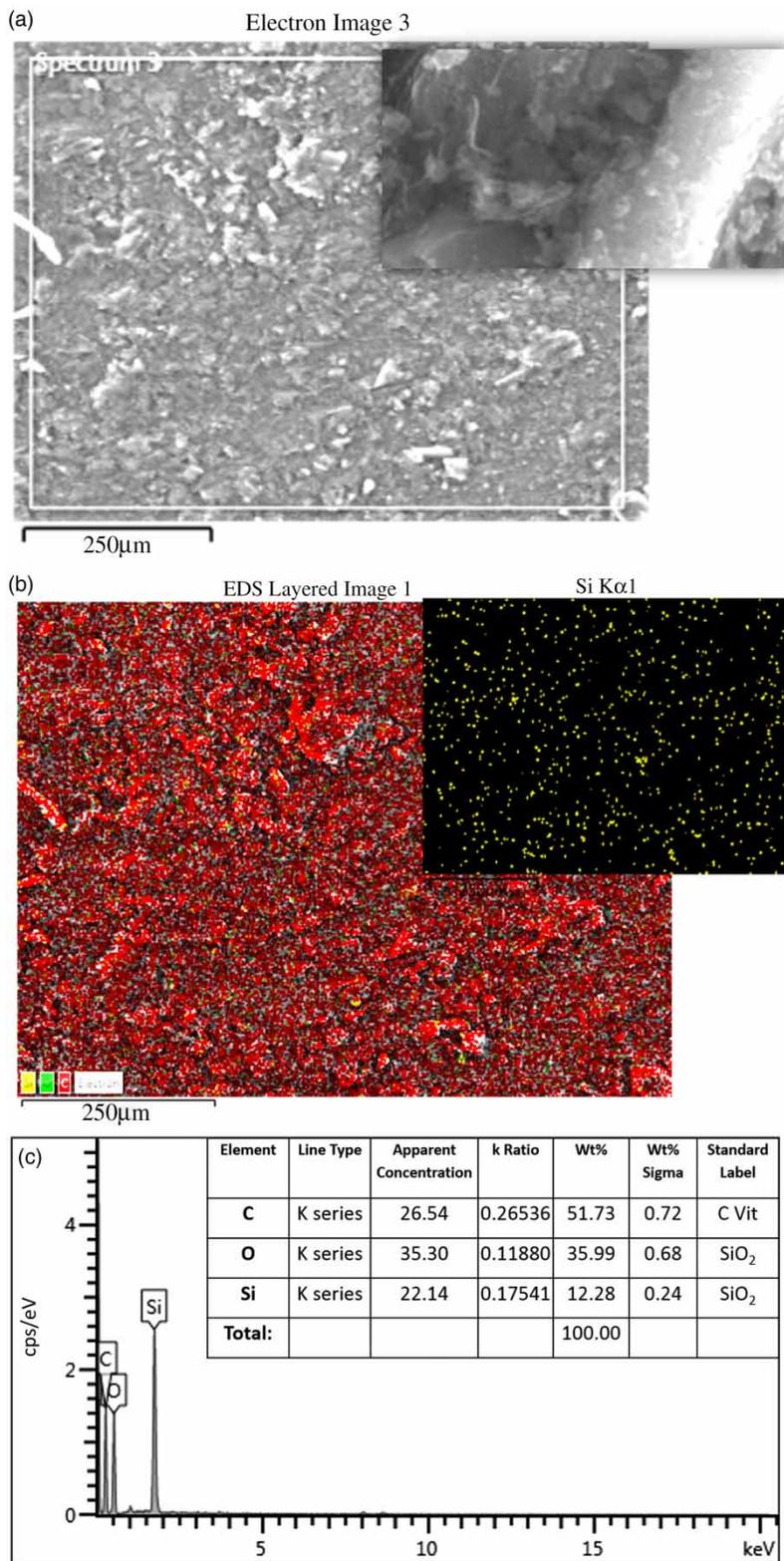
Figure 3 | SEM images, EDS mapping and EDX spectrum of silica/AC.
