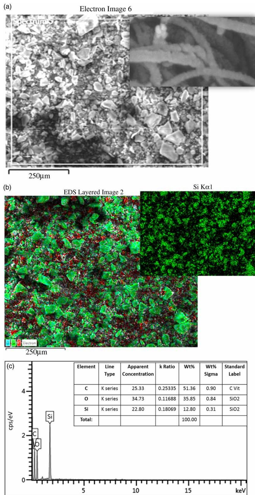
**Figure 2** | SEM images, energy dispersive X-ray spectroscopy for elemental mapping (EDS) mapping and EDX spectrum of silica/CNT.
