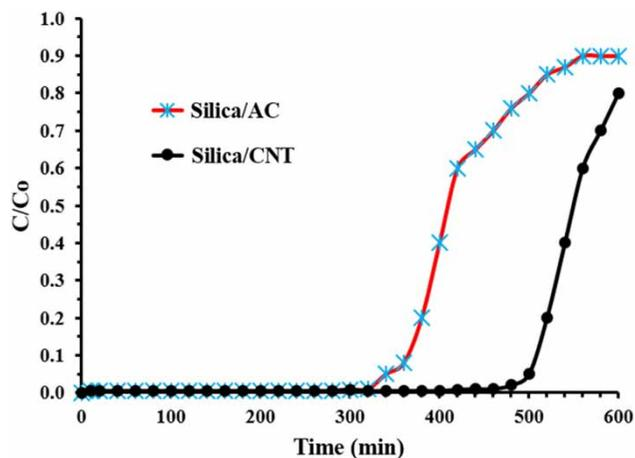
Figure 9 | Breakthrough curves of Hg<sup>2+</sup> on the silica/CNT and silica/AC.
