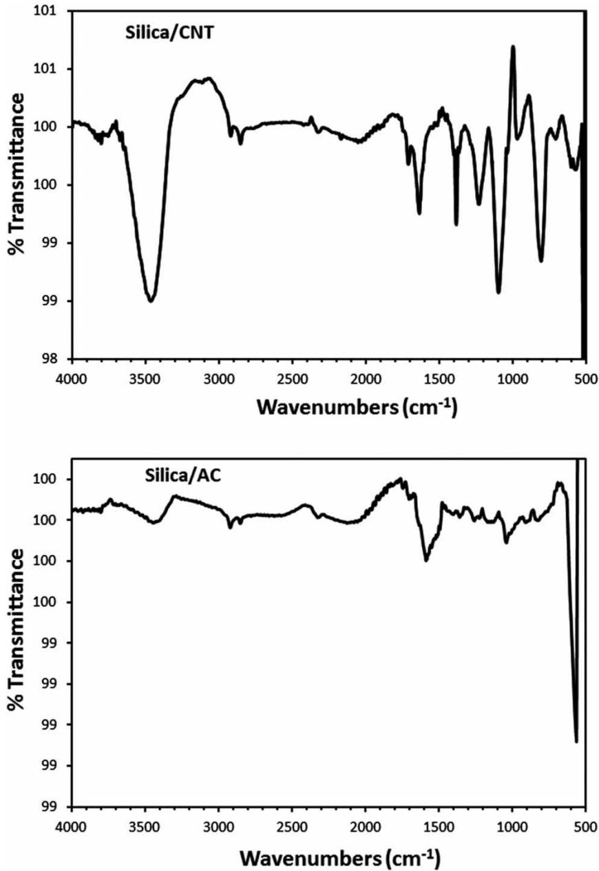
Figure 5 | FTIR spectrum of silica/CNT and silica/AC.
