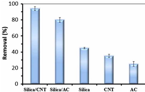
**Figure 6** | Comparison between AC, CNTs, silica, silica/AC and silica/CNT for Hg<sup>2+</sup> adsorption; initial concentrations of 40 ppm, dosage amounts 0.03 g, agitation speed 150 rpm, contact time 120 min.
