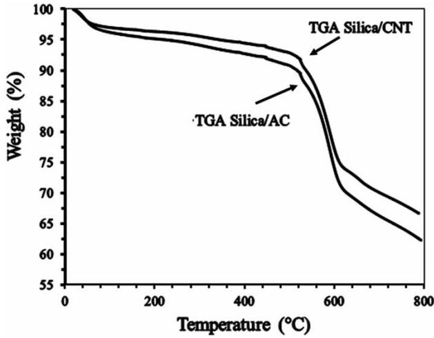
Figure 4 | TGA analysis of silica/CNT and silica/AC.
