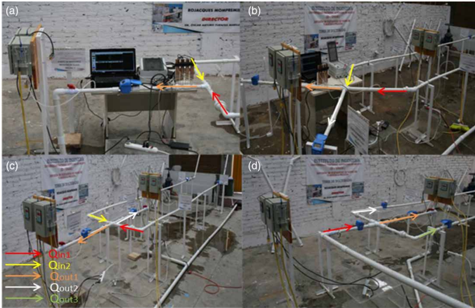
Figure 1 | Configurations of the experimental setup: (a) two inlets with one outlet; (b) two inlets at 90° with two outlets; (c) two inlets at 180° and two outlets; (d) one inlet and three outlets.
