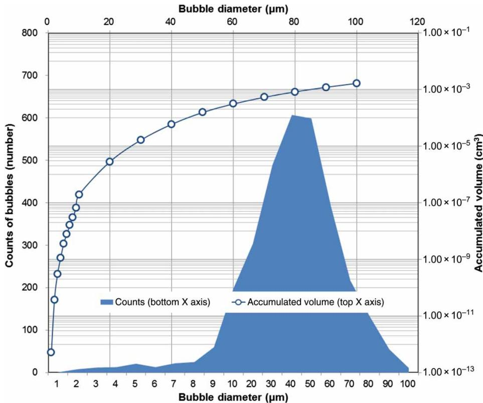
**Figure 7** | Bubble size distribution in terms of diameter of bubbles.
