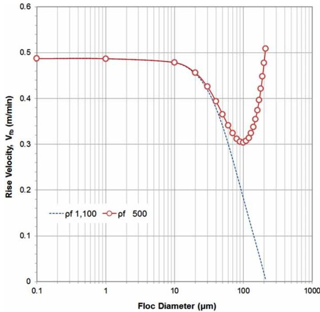
Figure 4 | Bubble-floc aggregate rise velocity depending on floc size for two initial floc densities 500 kg/m<sup>3</sup> and 1,100 kg/m<sup>3</sup>.
