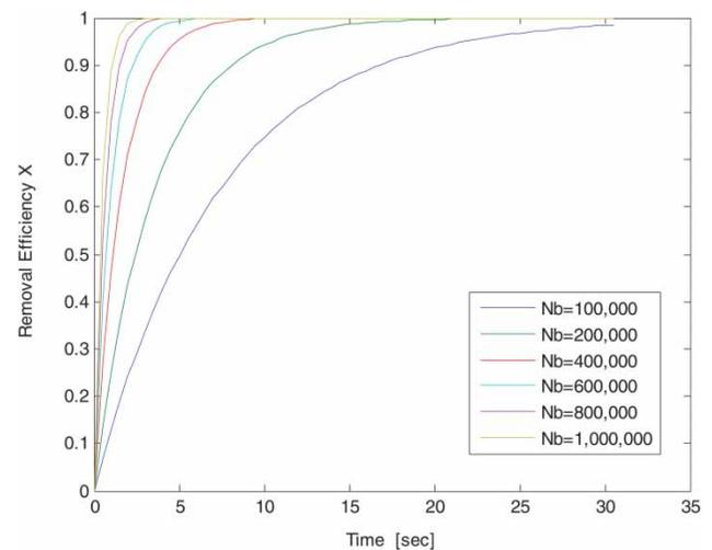
**Figure 5** | Removal efficiency of bubble-floc aggregates depending on the bubble number calculated by the PBT model.
