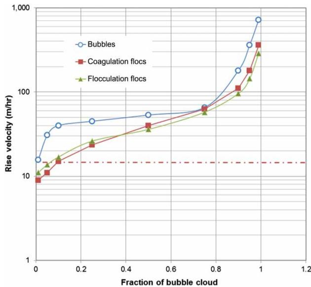
**Figure 8** | Rise velocity of bubbles and bubble-floc aggregates with change of bubble cloud bed depth.
