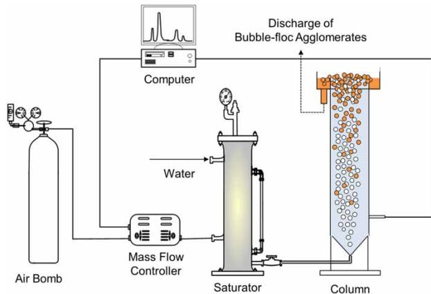
**Figure 1** | Schematic diagram of lab-scale pilot plant used in this study.
