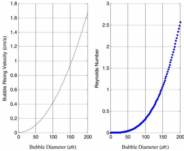
Figure 3 | Rise velocity of bubble and Reynolds number depending on bubble sizes.
