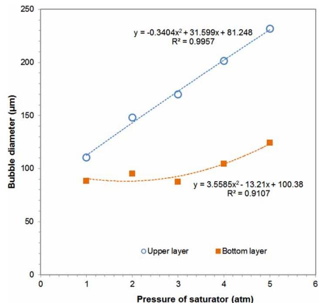
**Figure 2** | Bubble diameter change due to pressure formed in upper layer and bottom layer of the flotation cell.
