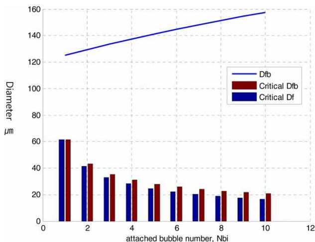
**Figure 6** | Critical bubble-floc aggregate diameter,  $Critical D_{fb}$ , and critical floc diameter,  $Critical D_f$ , related to attached bubble numbers (initial floc diameter = 250  $\mu\text{m}$ , bubble diameter = 120  $\mu\text{m}$ ,  $\rho_f$  900 <  $\rho_w$  1,000,  $D_{fb}$  = diameter of bubble-floc aggregate).
