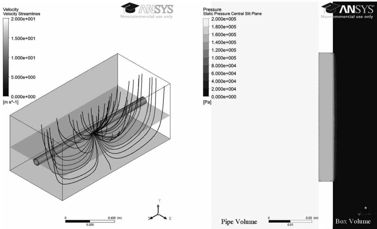
**Figure 3** | CFD simulation results for leak into porous media representative of gravel, from a  $60 \times 1$  mm longitudinal slit leaking into a fully submerged test section box. Velocity streamlines (left) and static pressure contour on central slit plane (right). Plane of interest shown as transparent surface on velocity streamline plot.
