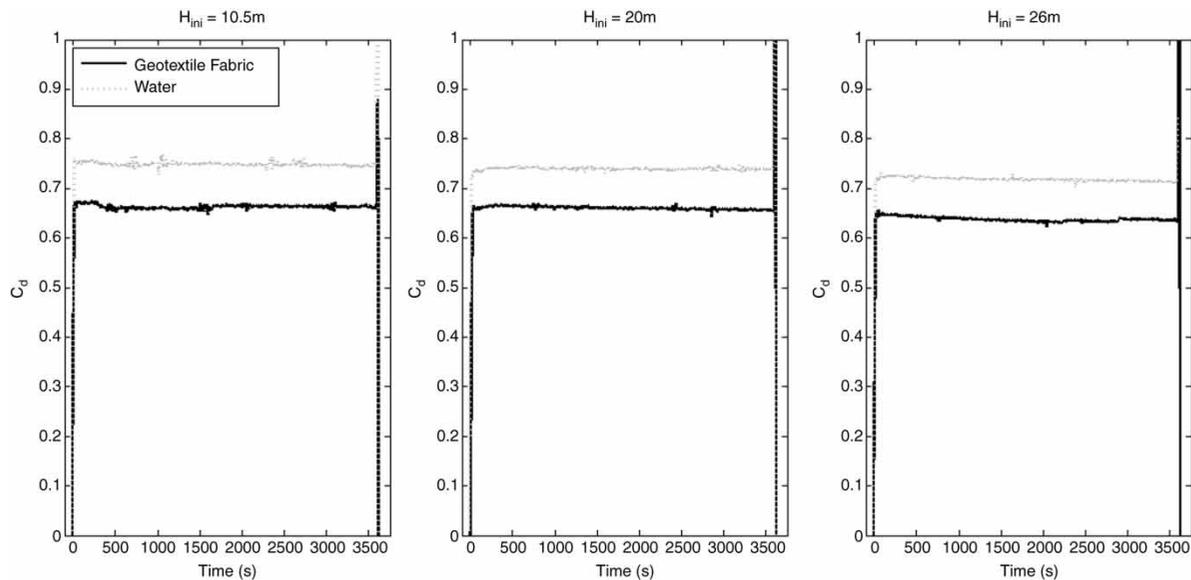
**Figure 7** | Time series of evaluated discharge coefficients ( $C_d$ ) for  $60 \times 1$  mm longitudinal slit in MDPE pipe at three discrete pressure heads for test cases into water (dotted line) and geotextile fabric (solid line).
