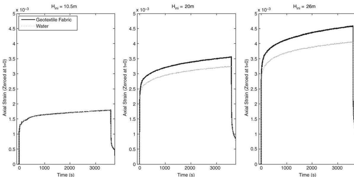
Figure 6 | Axial strain measured parallel to a  $60 \times 1$  mm longitudinal slit in MDPE pipe at three discrete pressure heads for test cases into water (dotted line) and geotextile fabric (solid line).
