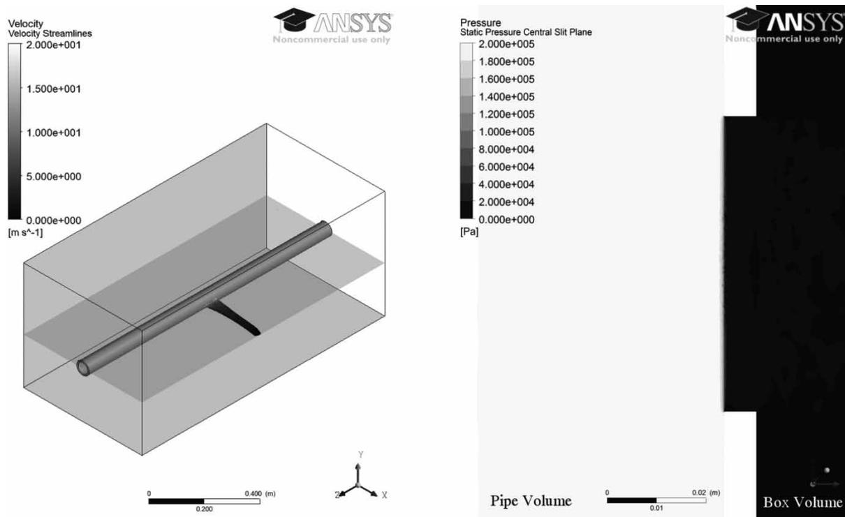
**Figure 2** | CFD simulation results for leak into water, from a  $60 \times 1$  mm longitudinal slit leaking into a fully submerged test section box. Velocity streamlines (left) and static pressure contour on central slit plane (right). Plane of interest shown as transparent surface on velocity streamline plot.
