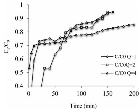
Figure 6 | Effect of flow rate on 4-chlorophenol adsorption.
