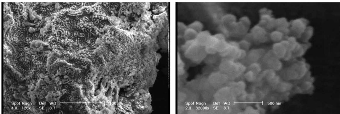
Figure 2 | SEM of nano graphene oxide.
