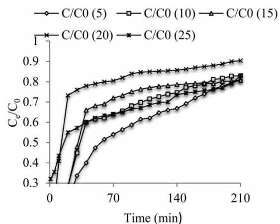
Figure 7 | Effect of initial concentration on time to exhaustion and adsorption capacity.
