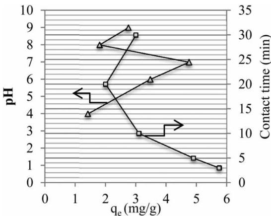
Figure 3 | Effect of pH and contact time on 4-chlorophenol adsorption rate.
