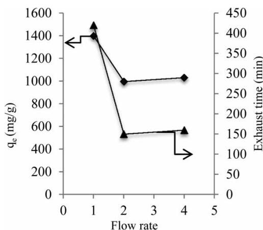
Figure 5 | Effect of flow rate on time to exhaustion and adsorption capacity.
