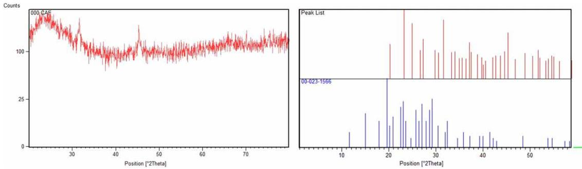
Figure 1 | X-ray diffraction of nano graphene oxide.
