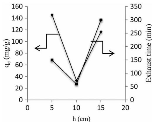
Figure 10 | Effect of bed depth on 4-chlorophenol adsorption.
