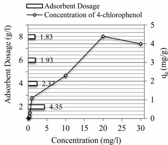
Figure 4 | Effect of dosage and initial concentration of 4-chlorophenol on adsorption.
