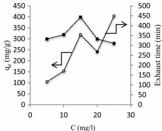
Figure 8 | Effect of initial concentration on 4-chlorophenol adsorption.
