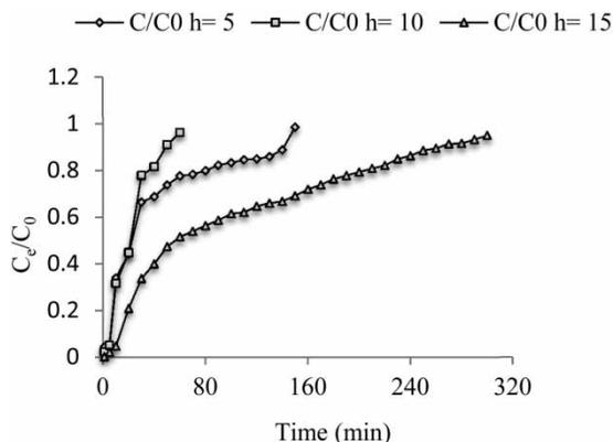
Figure 9 | Effect of bed depth on time to exhaustion and adsorption capacity.
