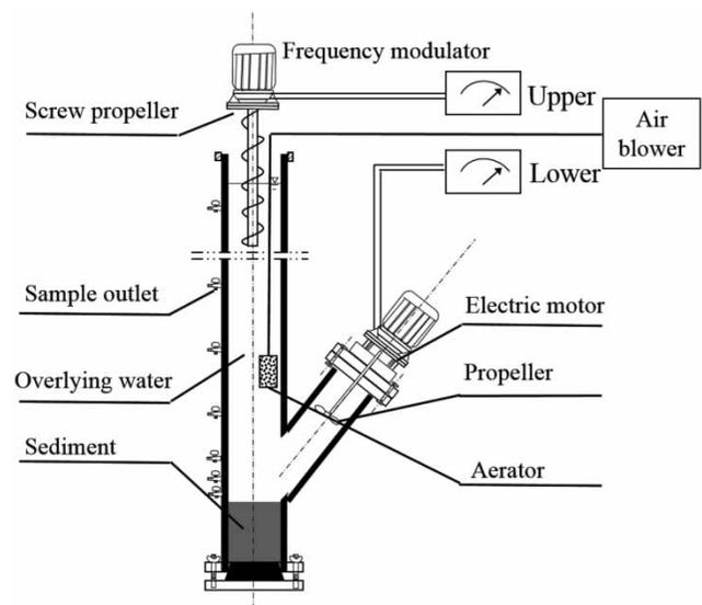
Figure 1 | Y-shaped sediment re-suspension generation apparatus.
