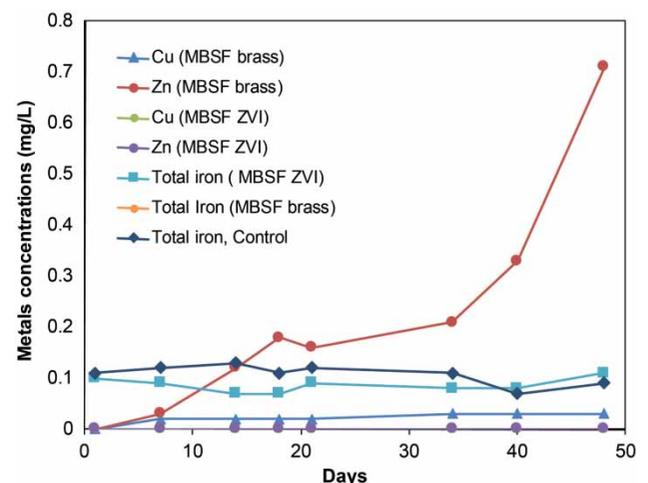
Figure 2 | Filter effluents metal concentrations.
