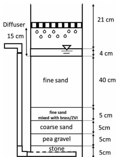
Figure 1 | Modified filter set up.
