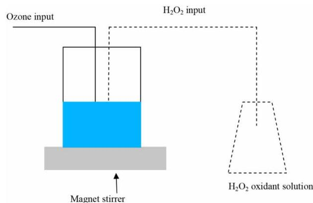
Figure 1 | Experimental set-up of the batch oxidation reactor.
