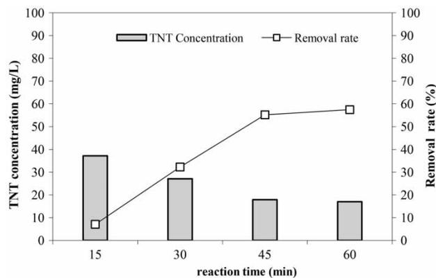
**Figure 9** | Effect of reaction time on TNT degradation ( $\text{H}_2\text{O}_2$  alone oxidation): TNT initial concentration = 40 mg/L, pH of solution = 10,  $\text{H}_2\text{O}_2/\text{TNT}$  molar ratio = 1,000:1.
