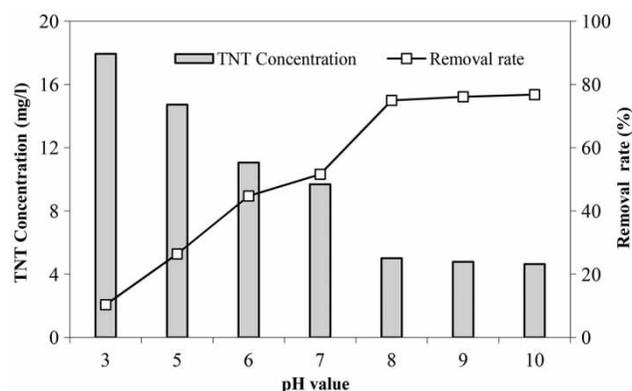
**Figure 2** | Effect of pH solution on TNT decomposition (simple ozonation): TNT initial concentration = 20 mg/L, dosage of ozone = 0.5 g/hr, reaction time = 30 min.
