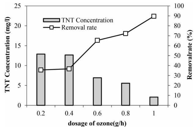
**Figure 6** | Effect of dosage of ozone on TNT degradation (simple ozonation): TNT concentration = 20 mg/L, pH of solution = 10, reaction time = 30 min.
