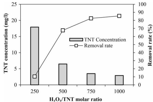
**Figure 7** | Effect of  $H_2O_2$ /TNT molar ratio on TNT degradation ( $H_2O_2$  oxidation): TNT concentration = 20 mg/L, pH of solution = 3, reaction time = 30 min.
