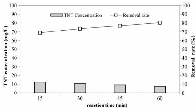
**Figure 8** | Effect of reaction time on TNT degradation (simple ozonation): TNT initial concentration = 40 mg/L, pH of solution = 10, dosage of ozone = 1 g/hr.
