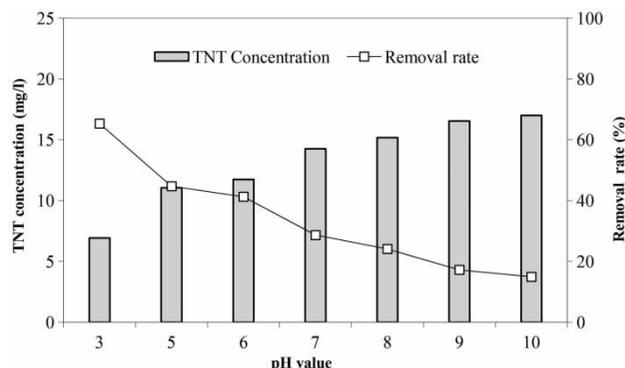
**Figure 3** | Effect of pH solution on TNT decomposition ( $\text{H}_2\text{O}_2$  oxidation): TNT initial concentration = 20 mg/L,  $\text{H}_2\text{O}_2/\text{TNT}$  molar ratio = 500:1, reaction time = 30 min.
