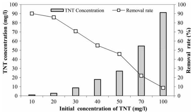
**Figure 5** | Effect of initial concentration on TNT degradation rate ( $H_2O_2$  alone oxidation): pH of solution = 3,  $H_2O_2$ /TNT molar ratio = 500:1, reaction time = 30 min.
