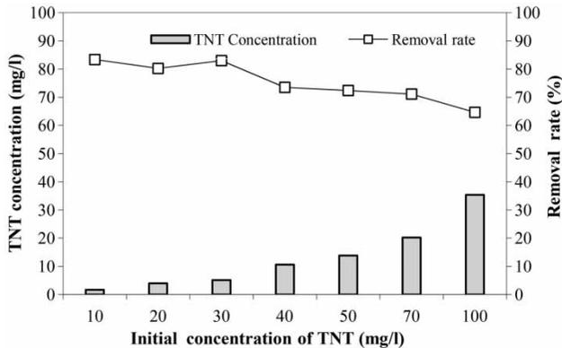
**Figure 4** | Effect of initial concentration on TNT degradation rate (simple ozonation): pH of solution = 10, dosage of ozone = 0.5 g/hr, reaction time = 30 min.
