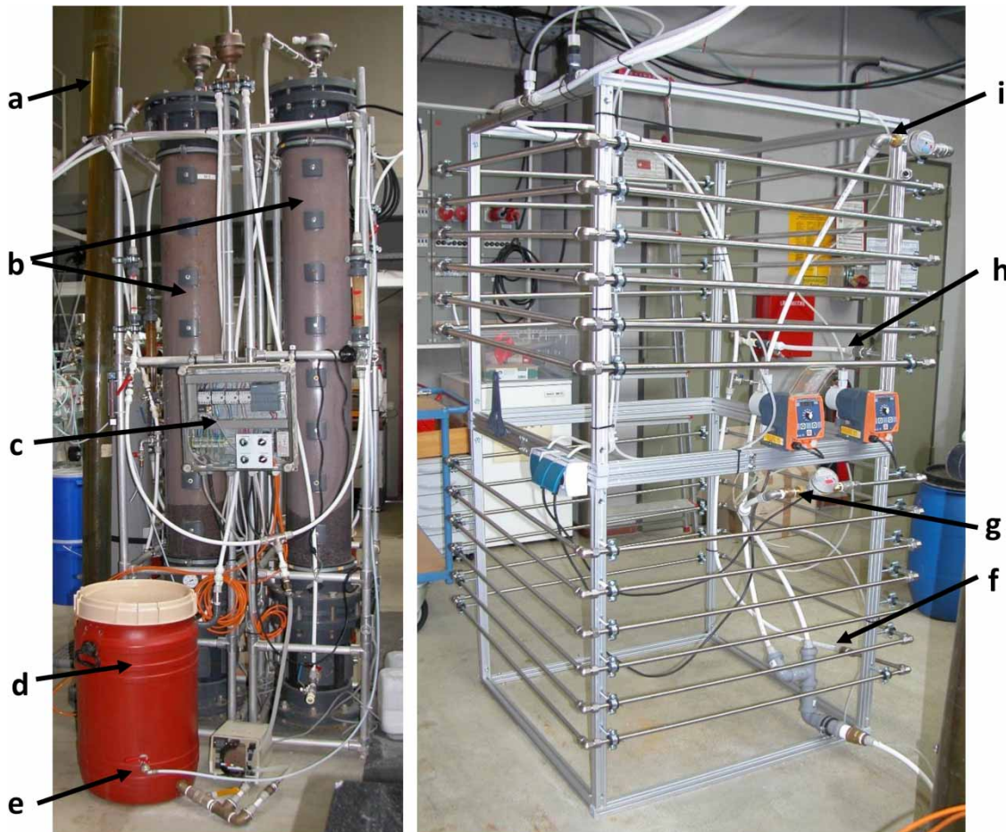
Figure 2 | Calcification plant for the generation of supersaturated water (left) and formation of solid calcite deposits in stainless steel pipes (right). CO 2 gassing column (a); filter columns with CaCO 3 (b); programmable logic controller PLC (c); storage tank with degassing unit (d); air inlet (e); inlet of supersaturated water into 10.0 mm stainless steel pipes (f); outlet of 10 mm stainless steel pipes with flow meter (g); inlet of supersaturated water into 15.7 mm stainless steel pipes (h); and outlet of 15.7 mm stainless steel pipes with flow meter (i).
