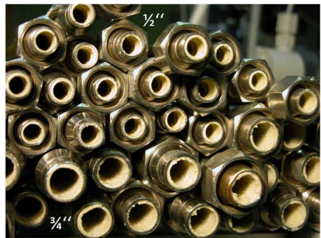
Figure 4 | Uniform and solid calcite layers inside stainless steel pipes with original 10 and 15.7 mm inner diameter (1/2" and 3/4", respectively) after precipitation process for about 69 days.
