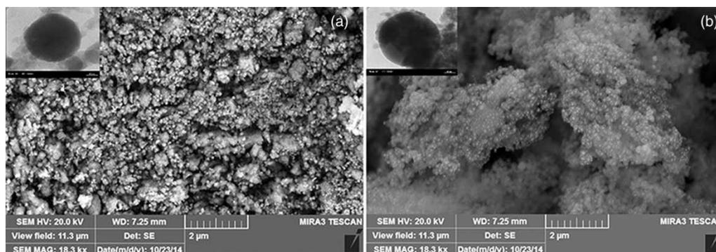
**Figure 6** | SEM and TEM (insets) images of (a) MNS and (b) AMNS nanospheres.
