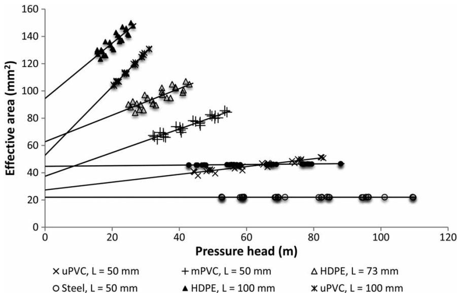
Figure 4 | Effective leak area against pressure head for longitudinal slits.
