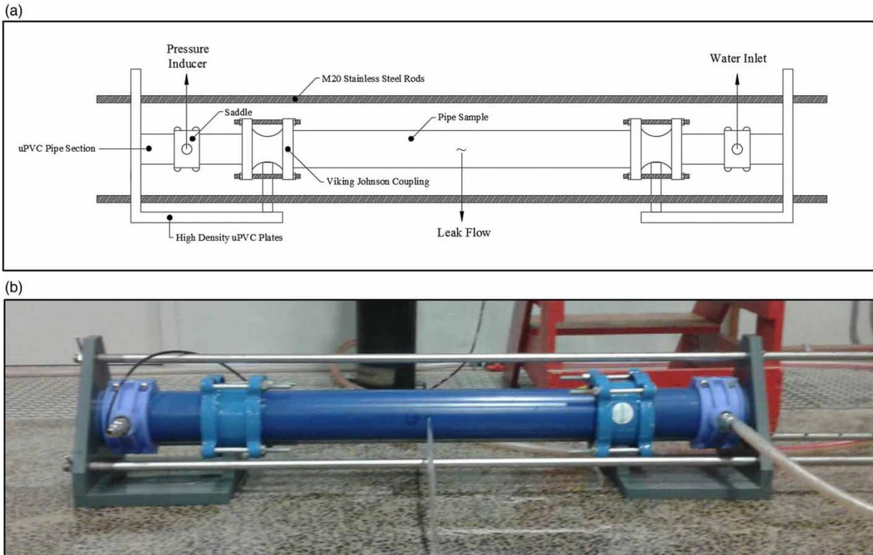
**Figure 1** | Schematic layout and photograph of the main components of the experimental setup.
