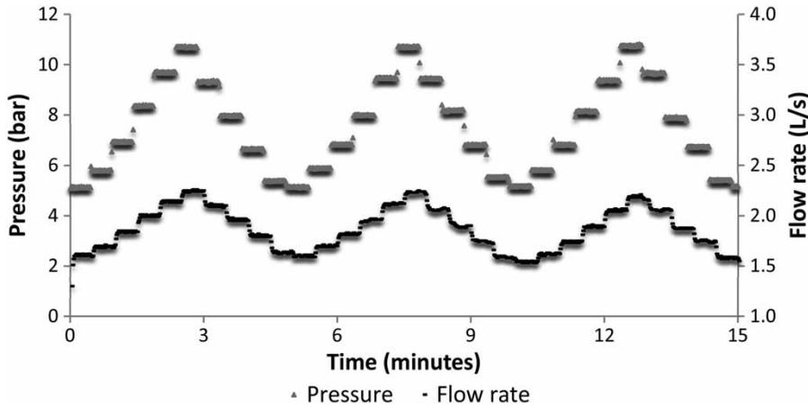
Figure 2 | Logged flow and pressure data for a typical experimental run.
