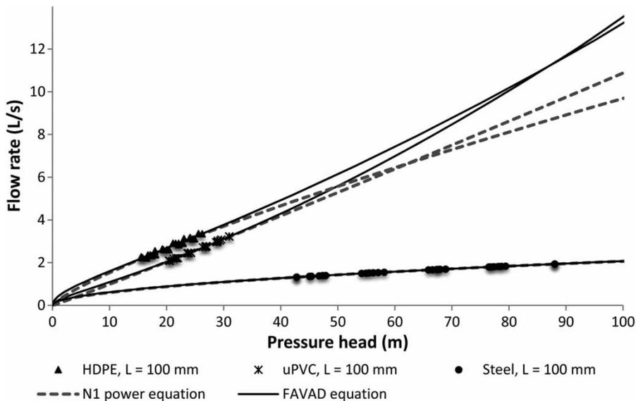
**Figure 7** | Comparison of the N1 power and FAVAD equation flow predictions for 100 mm slits in uPVC, HDPE and steel pipes.
