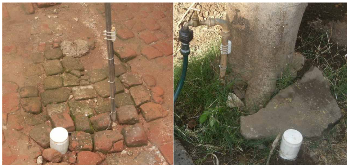
Figure 1 | Complete setup of recorder (in PVC casing) and microphone (covered by a block of PVC rubber) at the outdoor tap.
