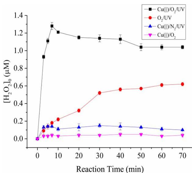
**Figure 4** | The concentrations of H<sub>2</sub>O<sub>2</sub> in the Cu(II)/O<sub>2</sub>, O<sub>2</sub>/UV, Cu(II)/O<sub>2</sub>/UV and Cu(II)/N<sub>2</sub>/UV processes. Experimental conditions: [Cu(II)]<sub>0</sub> = 50 μM, power of UV light = 15 W, O<sub>2</sub> flow rate = 0.5 L·min<sup>-1</sup>, pH = 3.5 ± 0.1, 20 °C, reaction time = 70 min.
