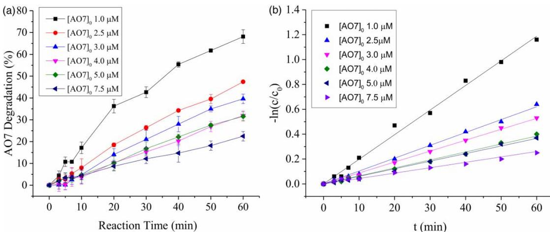
**Figure 10** | (a) Effect of dosage of AO7 on AO7 degradation in the Cu(II)/O<sub>2</sub>/UV process, and (b) linear fit of rate constants from kinetic models for the degradation of AO7 in the Cu(II)/O<sub>2</sub>/UV process. Experimental conditions: [Cu(II)]<sub>0</sub> = 10  $\mu\text{M}$ , [AO7]<sub>0</sub> = 1.0, 2.5, 3.0, 4.0, 5.0 and 7.5  $\mu\text{M}$ , O<sub>2</sub> flow rate = 0.5 L·min<sup>-1</sup>, power of UV light = 15 W, pH = 3.5 ± 0.1, 20 °C, reaction time = 60 min.
