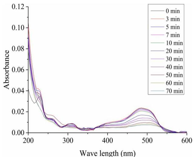
**Figure 12** | The UV full scan in the Cu(II)/O<sub>2</sub>/UV process. Experimental conditions: [Cu(II)]<sub>0</sub> = 10 μM, [AO7]<sub>0</sub> = 1.5 μM, power of UV light = 15 W, O<sub>2</sub> flow rate = 0.5 L·min<sup>-1</sup>, pH = 3.5 ± 0.1, 20 °C, reaction time = 70 min.
