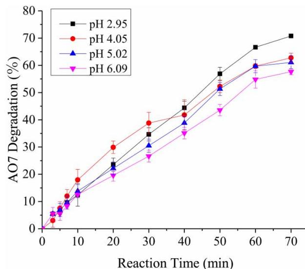
**Figure 7** | Effect of pH on the degradation of AO7 in the Cu(II)/ $\text{O}_2$ /UV process. Experimental conditions:  $[\text{Cu(II)}]_0 = 10 \mu\text{M}$ ,  $[\text{AO7}]_0 = 1.5 \mu\text{M}$ , power of UV light = 15 W,  $\text{O}_2$  flow rate =  $0.5 \text{ L}\cdot\text{min}^{-1}$ ,  $\text{pH} = 2.95, 4.05, 5.02$  and  $6.09$ ,  $20^\circ\text{C}$ , reaction time = 70 min.
