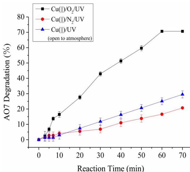
**Figure 5** | The role of O<sub>2</sub> in the Cu(II)/O<sub>2</sub>/UV process. Experimental conditions: [Cu(II)]<sub>0</sub> = 10 μM, [AO7]<sub>0</sub> = 1.5 μM, power of UV light = 15 W, O<sub>2</sub> flow rate = 0.5 L·min<sup>-1</sup>, N<sub>2</sub> flow rate = 0.5 L·min<sup>-1</sup>, pH = 3.5 ± 0.1, 20 °C, reaction time = 70 min.
