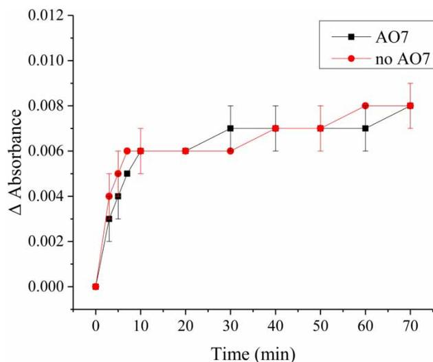
**Figure 3** | Change of the absorbance of DPA in the Cu(II)/O<sub>2</sub>/UV with AO7 and without AO7 processes. Experimental conditions: [Cu(II)]<sub>0</sub> = 10 μM, [AO7]<sub>0</sub> = 1.5 μM, [DPA]<sub>0</sub> = 2.0 μM, power of UV light = 15 W, O<sub>2</sub> flow rate = 0.5 L·min<sup>-1</sup>, pH = 3.5 ± 0.1, 20 °C, reaction time = 70 min.
