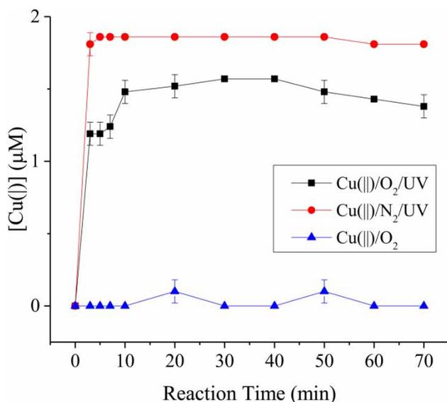
**Figure 6** | The concentrations of Cu(I) in the Cu(II)/ $\text{O}_2$ , Cu(II)/ $\text{O}_2$ /UV and Cu(II)/ $\text{N}_2$ /UV processes. Experimental conditions:  $[\text{Cu(II)}]_0 = 50 \mu\text{M}$ , power of UV light = 15 W,  $\text{O}_2$  flow rate =  $0.5 \text{ L}\cdot\text{min}^{-1}$ ,  $\text{N}_2$  flow rate =  $0.5 \text{ L}\cdot\text{min}^{-1}$ ,  $\text{pH} = 3.5 \pm 0.1$ ,  $20^\circ\text{C}$ , reaction time = 70 min.
