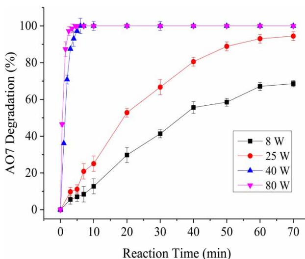
**Figure 9** | Effect of power of UV light on the degradation of AO7 in the Cu(II)/O<sub>2</sub>/UV process. Experimental conditions: [Cu(II)]<sub>0</sub> = 10 μM, [AO7]<sub>0</sub> = 1.5 μM, O<sub>2</sub> flow rate = 0.5 L·min<sup>-1</sup>, power of UV light = 8, 25, 40 and 80 W, pH = 3.5 ± 0.1, 20 °C, reaction time = 70 min.
