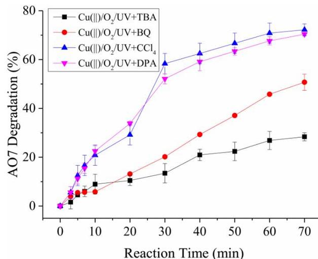
**Figure 2** | Effect of the addition of different radical scavengers on AO7 degradation in the  $Cu(II)/O_2/UV$  process. Experimental conditions:  $[Cu(II)]_0 = 10 \mu M$ ,  $[AO7]_0 = 1.5 \mu M$ ,  $[TBA]_0 = 25 mM$ ,  $[BQ]_0 = 0.15 mM$ ,  $[DPA]_0 = 2.0 \mu M$ , power of UV light = 15 W,  $O_2$  flow rate =  $0.5 L \cdot min^{-1}$ ,  $pH = 3.5 \pm 0.1$ ,  $20^\circ C$ , reaction time = 70 min.
