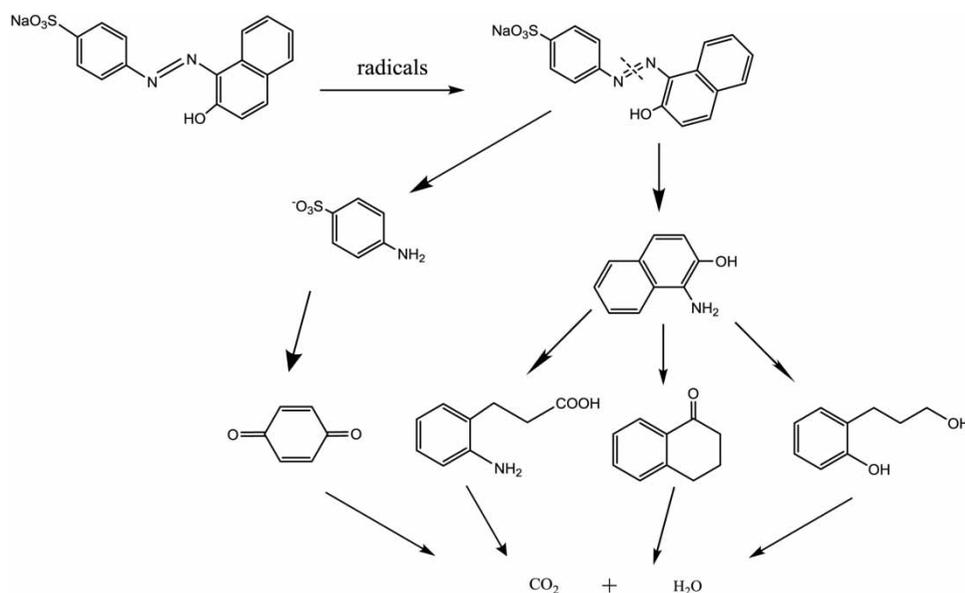
**Figure 13** | The degradation process of AO7 in the Cu(II)/O<sub>2</sub>/UV process.
