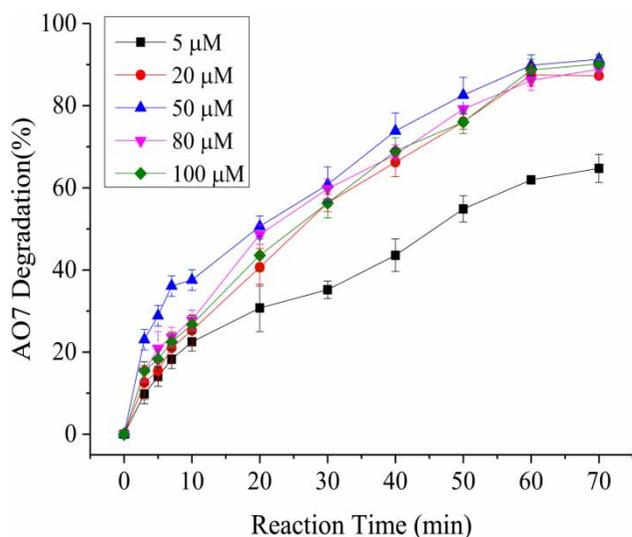
**Figure 8** | Effect of dosage of Cu(II) on the degradation of AO7 in the Cu(II)/O<sub>2</sub>/UV process. Experimental conditions: [Cu(II)]<sub>0</sub> = 5, 20, 50, 80 and 100 μM, [AO7]<sub>0</sub> = 1.5 μM, power of UV light = 15 W, O<sub>2</sub> flow rate = 0.5 L·min<sup>-1</sup>, pH = 3.5 ± 0.1, 20 °C, reaction time = 70 min.
