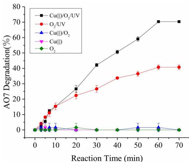
**Figure 1** | Time-dependent degradation of AO7 by  $O_2$ ,  $Cu(II)$ ,  $Cu(II)/O_2$ ,  $UV/O_2$  and  $Cu(II)/O_2/UV$  processes. Experimental conditions:  $[Cu(II)]_0 = 10 \mu M$ ,  $[AO7]_0 = 1.5 \mu M$ , power of UV light = 15 W,  $O_2$  flow rate =  $0.5 L \cdot min^{-1}$ ,  $pH = 3.5 \pm 0.1$ ,  $20^\circ C$ , reaction time = 70 min.
