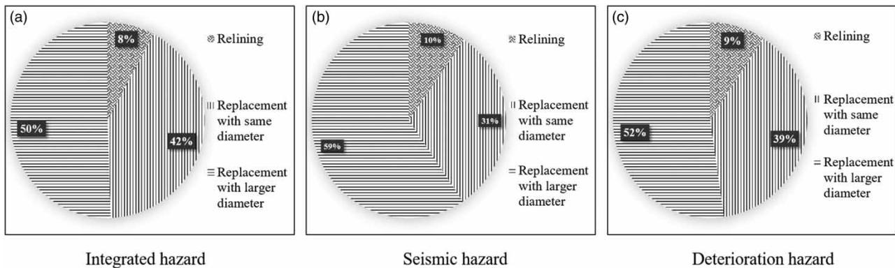
Figure 8 | Budget spent on different rehabilitation actions.
