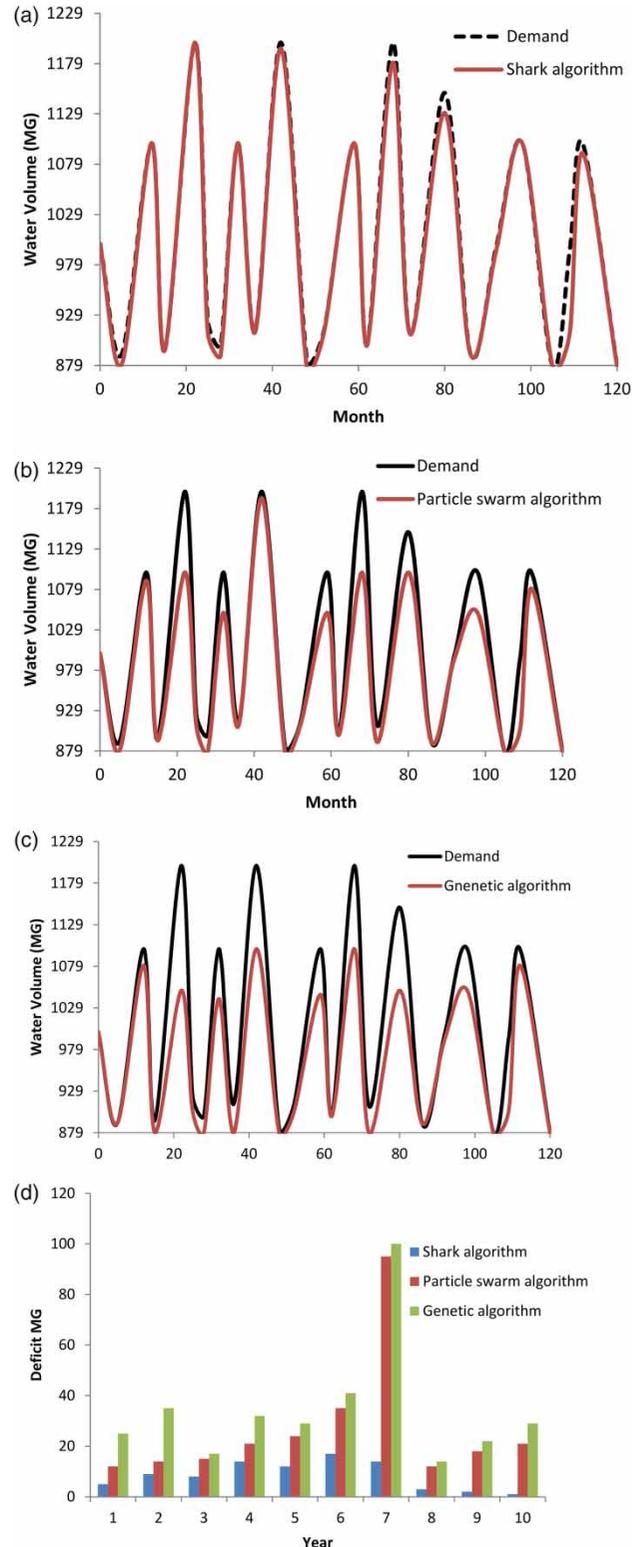
**Figure 5** | Release and demand analysis using historical inflow: (a) shark algorithm, (b) particle swarm algorithm, (c) genetic algorithm, (d) annual deficit (1994–2003).
