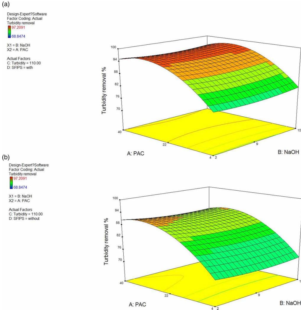
**Figure 4** | Response surface plots of turbidity removal as a function of PAC and  $Tur_{in}$  at a mean level of NaOH (8.5 mg/l) (a) with SFIPS and (b) without SFIPS; (c) plot of predicted vs. actual values for turbidity removal; (d) interactive effects of PAC-SFIPS on turbidity removal at a NaOH dose and  $Tur_{in}$  of 8.5 mg/l and 200 NTU, respectively (*Continued*.)
