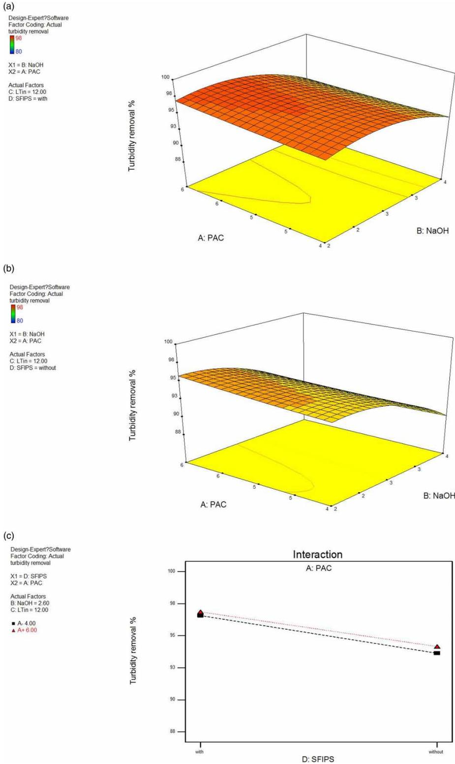
**Figure 3** | Response surface plots for turbidity removal as a function of PAC and NaOH at Tur<sub>in</sub> of 12 NTU (a) with SFIPS and (b) without SFIPS; (c) interactive effects of PAC-SFIPS on turbidity removal at a NaOH dose and Tur<sub>in</sub> of 2.6 mg/l and 12 NTU, respectively; (d) interactive effects of NaOH-SFIPS on turbidity removal at a PAC dose and Tur<sub>in</sub> of 5 mg/l and 12 NTU, respectively; (e) plot of predicted vs. actual values for turbidity removal. (Continued.)
