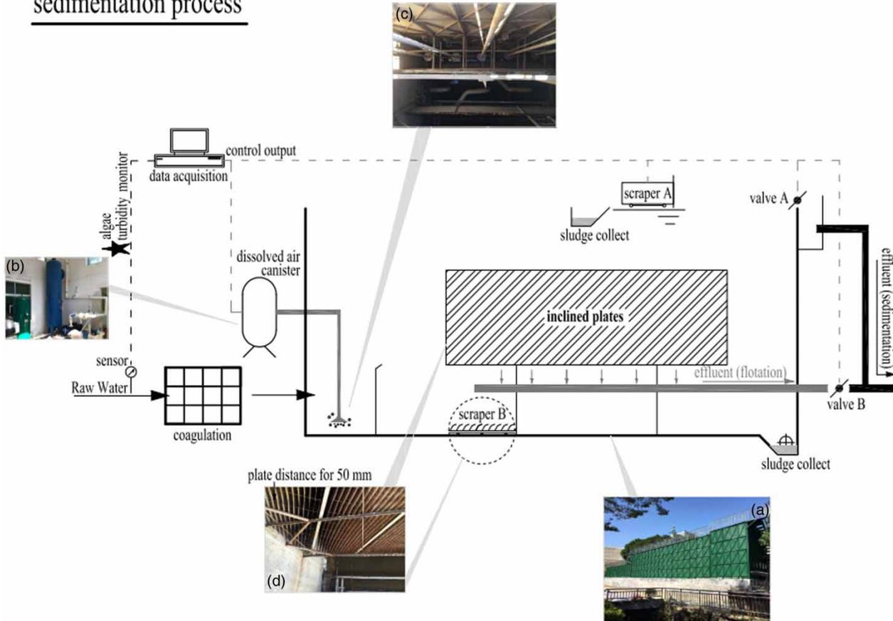
**Figure 1** | Flow diagram of the integrated flotation and sedimentation unit (IFSU). Thumbnail (a) shows the exterior of the IFSU, (b) is a snapshot of the dissolved air canister, (c) is a close-up view of the DAF releaser and (d) displays the side flow-inclined plates and scraper.
