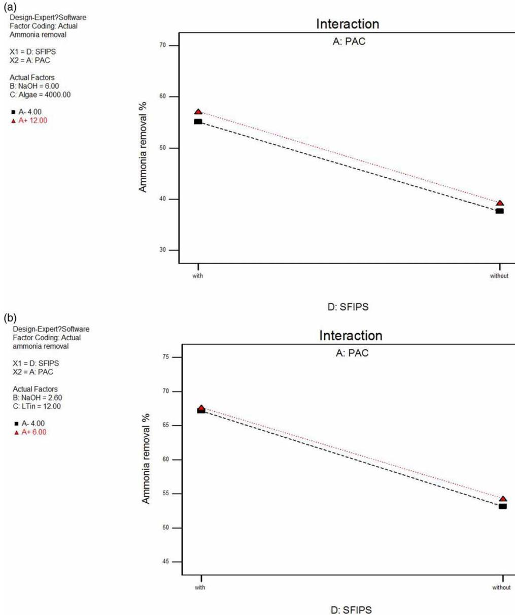
**Figure 6** | (a) Interactive effects of PAC-SFIPS on  $\text{NH}_4\text{-N}$  removal during treatment of algal-rich water at a NaOH dose and  $\text{Chl}_{in}$  of 6.0 mg/l and 4,000 mg/l, respectively; (b) interactive effects of PAC-SFIPS on  $\text{NH}_4\text{-N}$  removal during treatment of low-turbidity water at a NaOH dose and  $\text{Tur}_{in}$  of 2.6 mg/l and 12 NTU, respectively.
