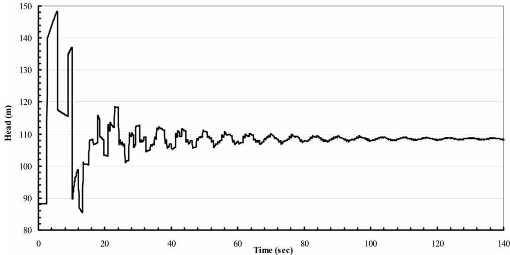
Figure 4 | Pressure head variation with time at a selected node (upstream of the valve) for FSP operation.
