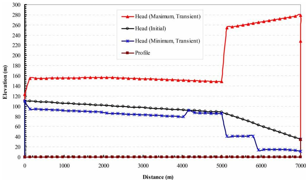
Figure 5 | Transient pressure heads enveloped due to valve sudden closure and using FSPs.
