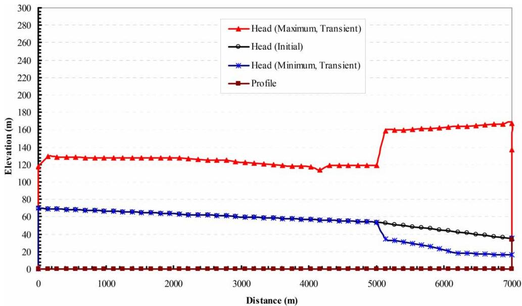
**Figure 7** | Transient pressure heads enveloped due to valve sudden closure and using VSPs.
