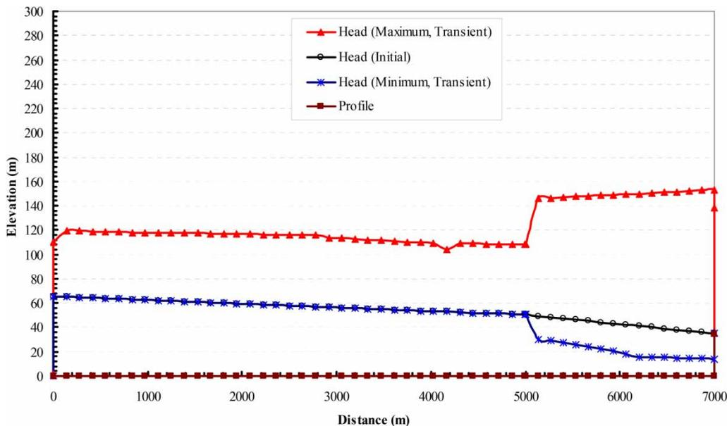
**Figure 9** | Transient pressure heads enveloped due to valve sudden closure at using VSPs and leakage is considered.
