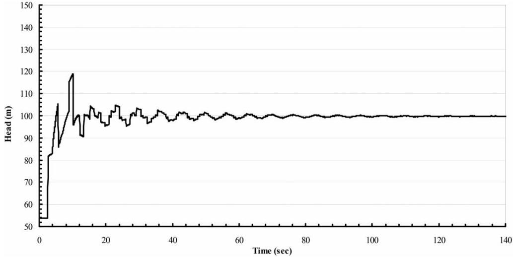
**Figure 6** | Pressure head variation with time at a selected node (upstream the valve) for VSP operation.
