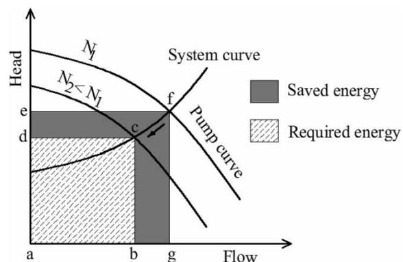
Figure 1 | Energy saved by using variable speed pumps (grey area).
