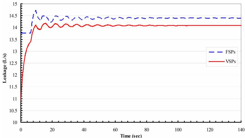
**Figure 10** | Variations of total leakage from the network with time and valve sudden closure.
