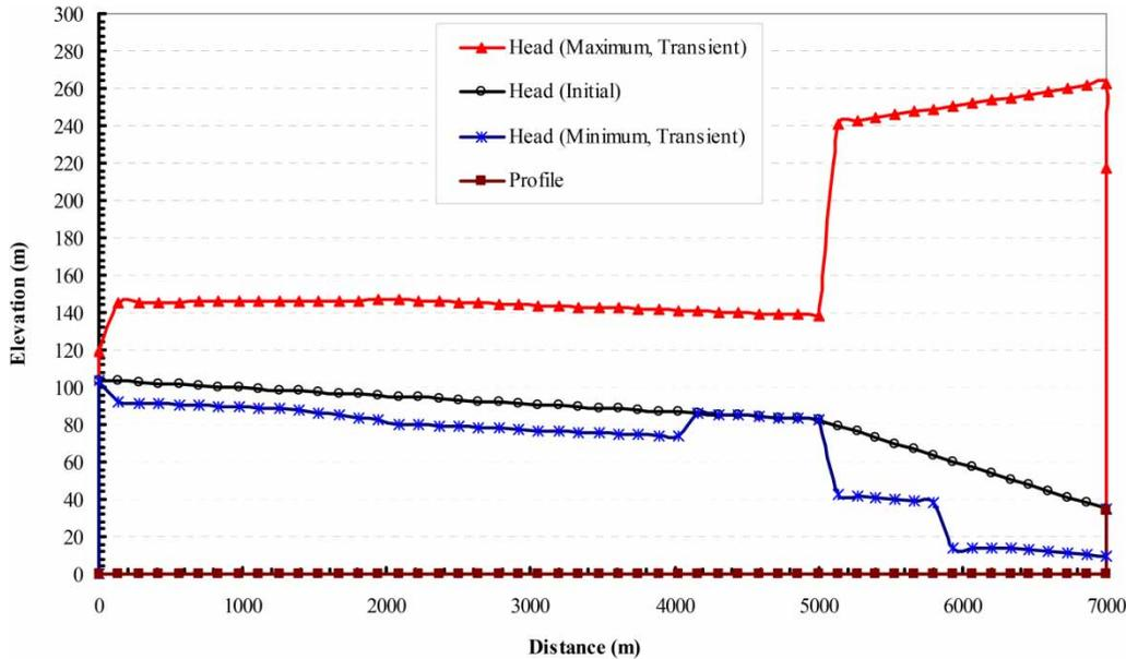
**Figure 8** | Transient pressure heads enveloped due to valve sudden closure at using FSPs and leakage is considered.
