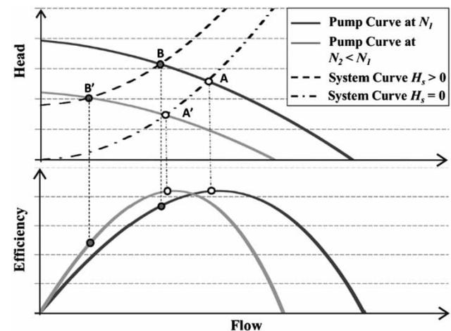
Figure 2 | Operating points and efficiencies with varying speeds in systems with and without static head (adapted from Marchi *et al.* 2012).
