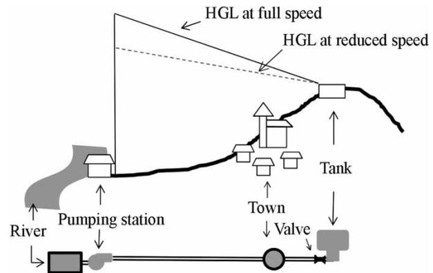
**Figure 3** | Case study layout and its EPANET representation (modified from [Marchi et al. 2012](#)).
